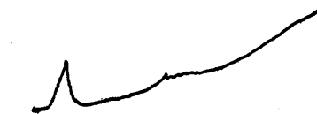
Fig. 16. Minutes oscillation due to local short circuit of transformer winding.
