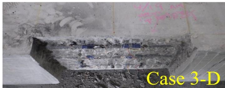
(c) Model beam with spalling of bottom concrete cover and section reduced in stirrups rebar
