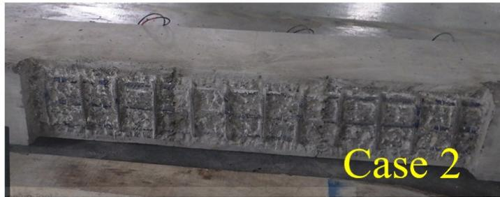
(b) Model beam with sectional defect in bottom concrete cover or rebars were exposed
