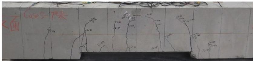
(b) Crack pattern of Case 2 after testing
