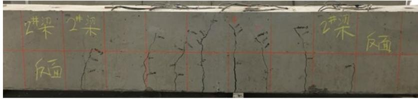
(a) Crack pattern of Case 1 after testing
