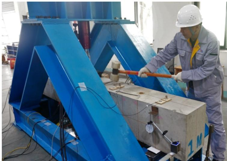
Fig. 4.7 The image of Impact Vibration Test
