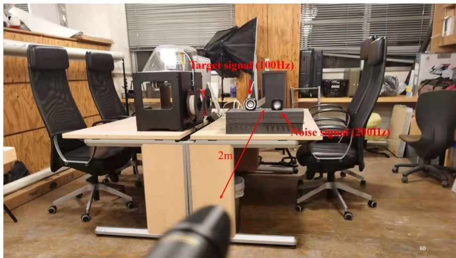
Figure 4.31 Experiment of extracting target signal in noise environment using microphone.
