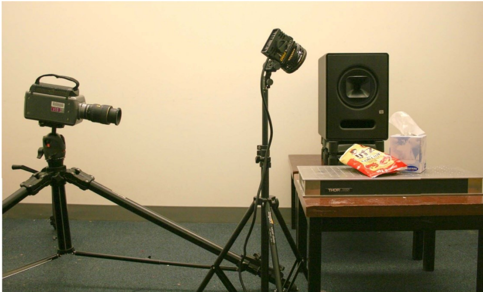
Figure 1.4 Example of experiment setup of Visual Microphone from MIT
