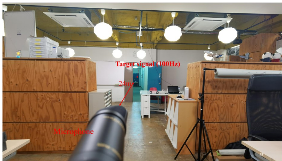
Figure 4.29 Experiment of extracting audio signal at long distance using electric microphone.
