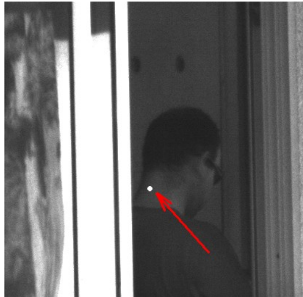
Figure 1.6 Listening to talks from the back part of the neck using laser speckle images
