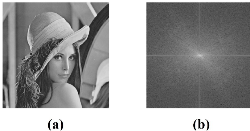
Figure 3.7 The Lenna image and its Fourier transform result. (a) Image in time domain (b) Image in frequency domain
