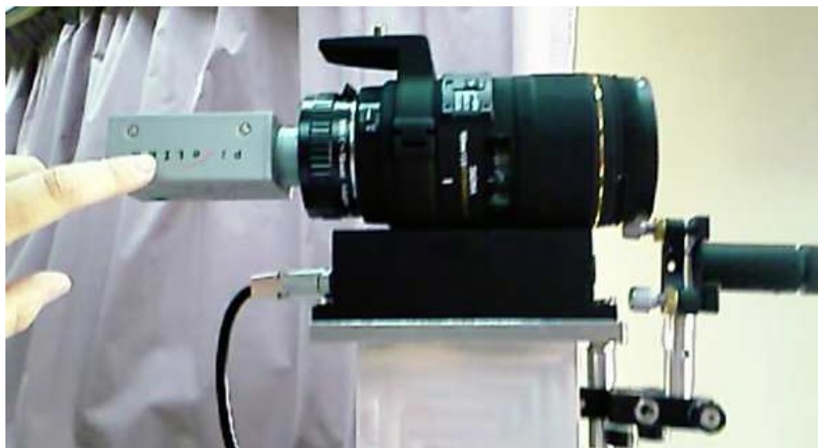
Figure 1.7 The experimental setups for far range detection using laser speckle images
