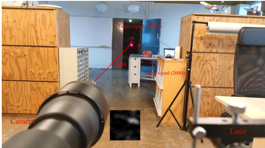
Figure 4.33 Experiment of extracting audio signal at long distance with noise in the environment using laser speckle images.
