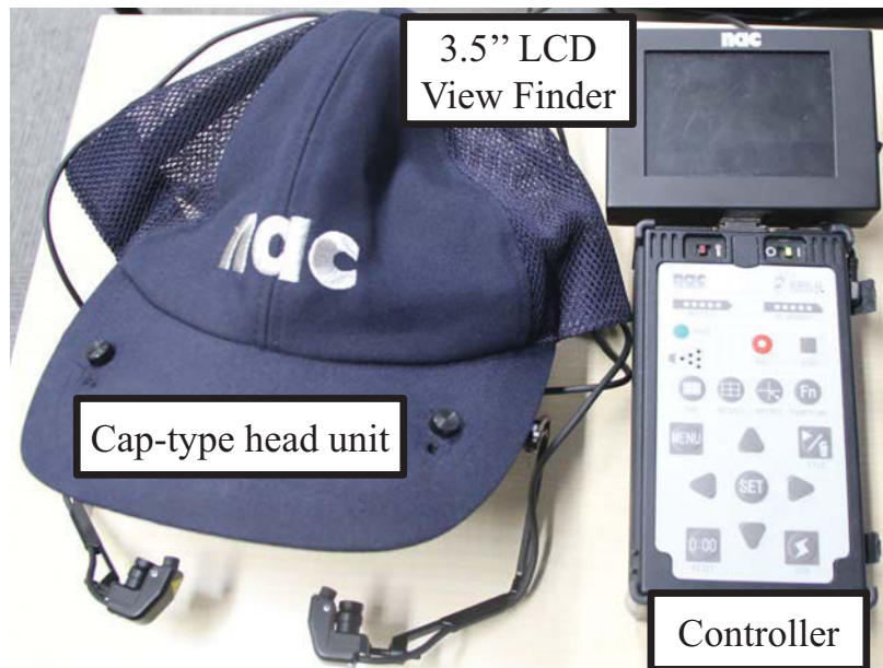
Figure 3-10: The eye-tracking device. The eye-tracking device (nac, EMR-9)
