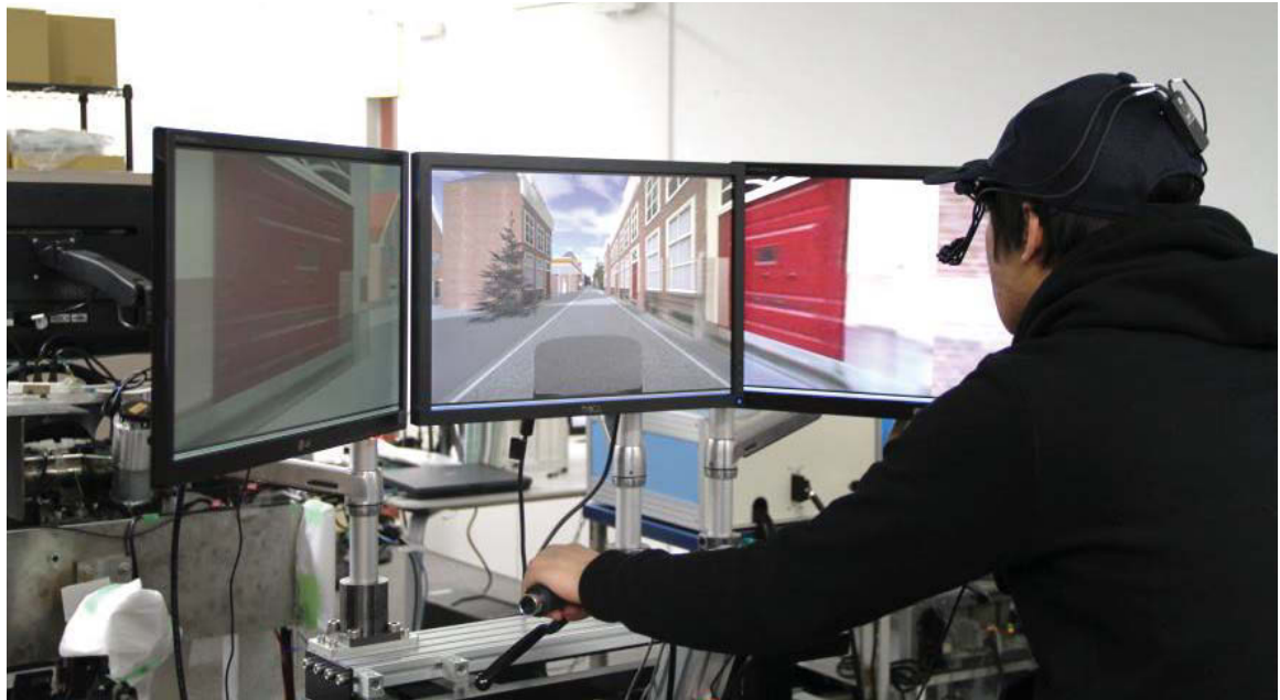
Figure 3-17: Non-immersive motorcycle simulator experiment scenery.
