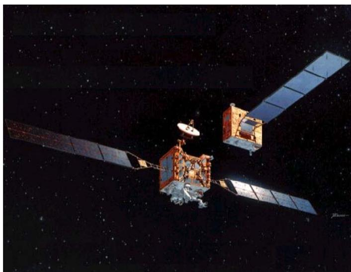
Fig. 3-1 Engineering Test Satellite VII (ETS-VII)
