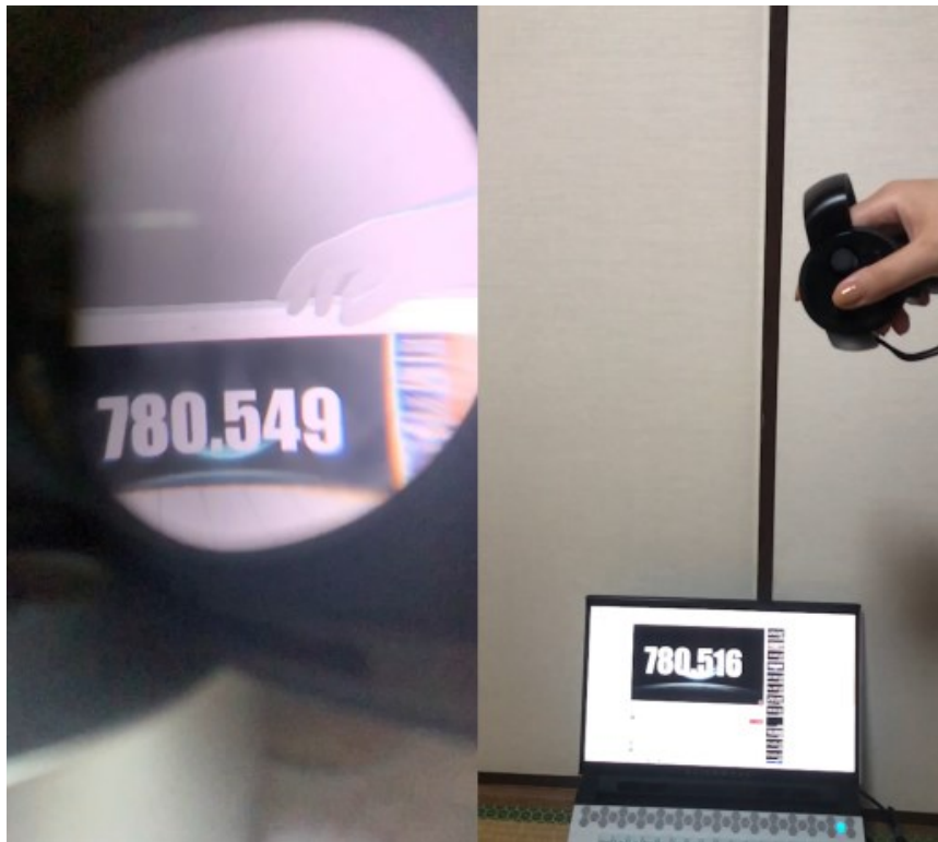
Figure 5.2 VR latency measurement
