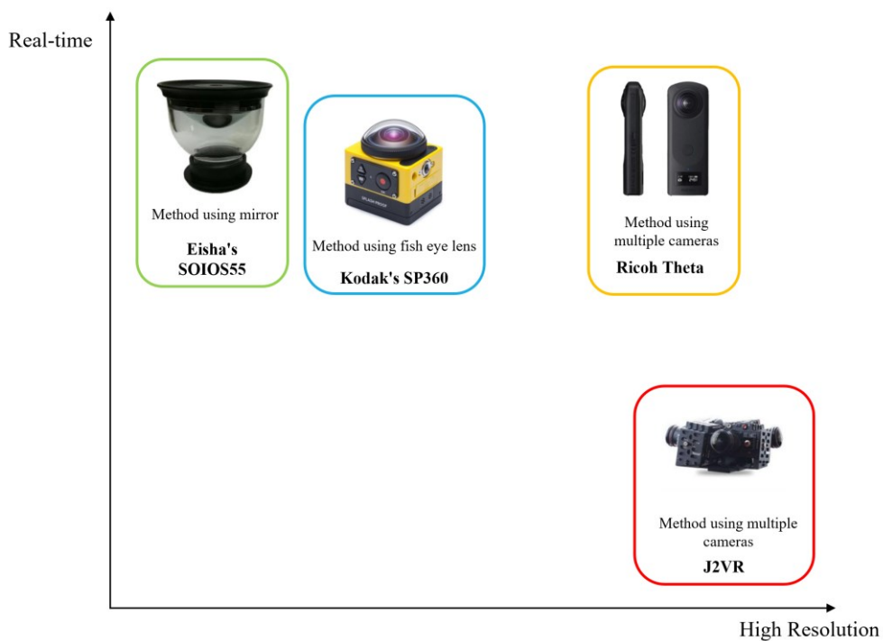
Figure 3. 7: characteristics of various types of 360-degree cameras
