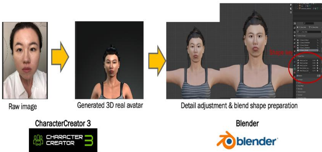
Figure 3-10 The process of creating a photorealistic avatar
