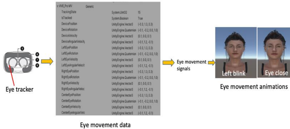
Figure 3-14 The process of simulating eye movement
