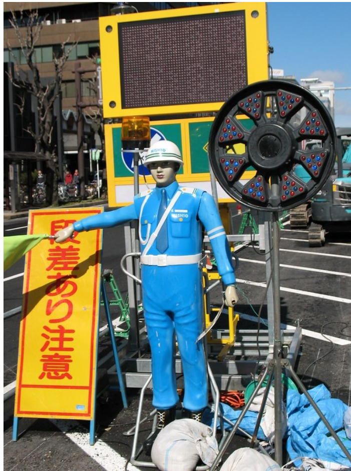
Figure 2-5 Example of temporary traffic control robot in Japan
