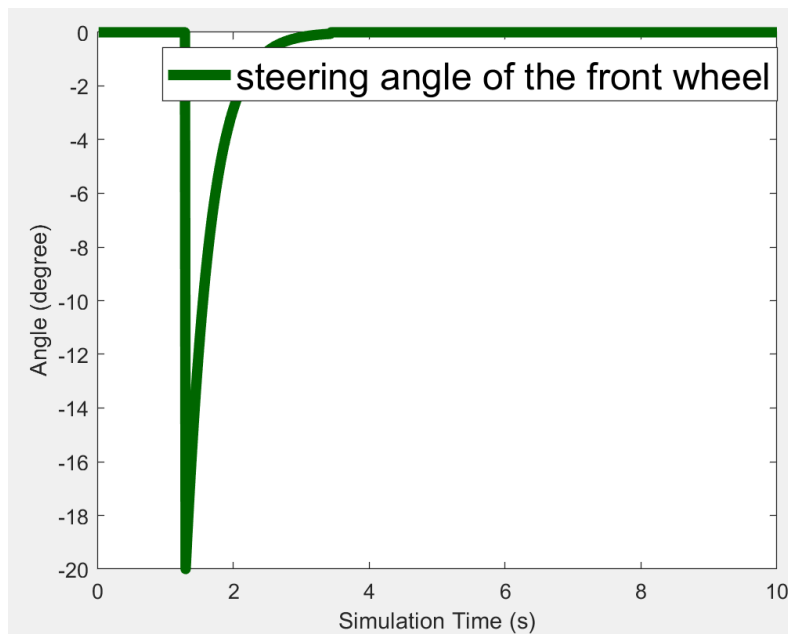
Figure 5-4 Steering Angel of the Front Wheel of Ego Vehicle
