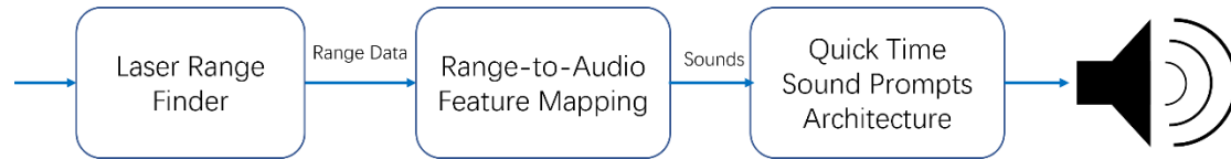
Figure 2.3 The System Structure with Laser Range Finder [13]
