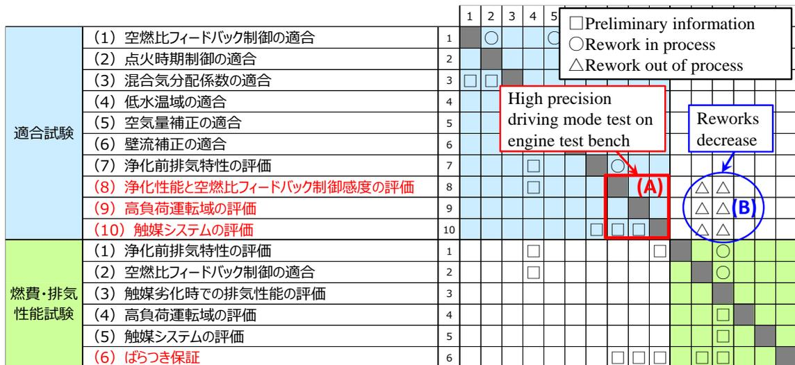
Fig. 3-12 Reduction of rework by high precision driving mode
