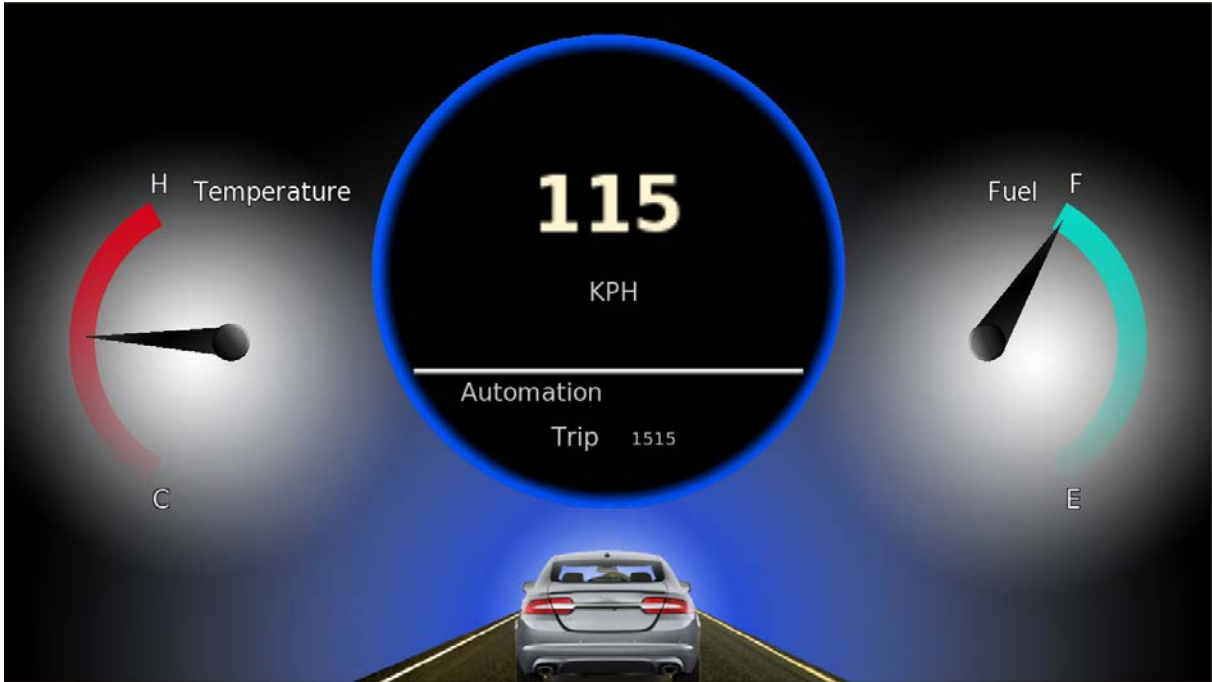
Figure 3.12 Cluster user interface created using SCADE Display
