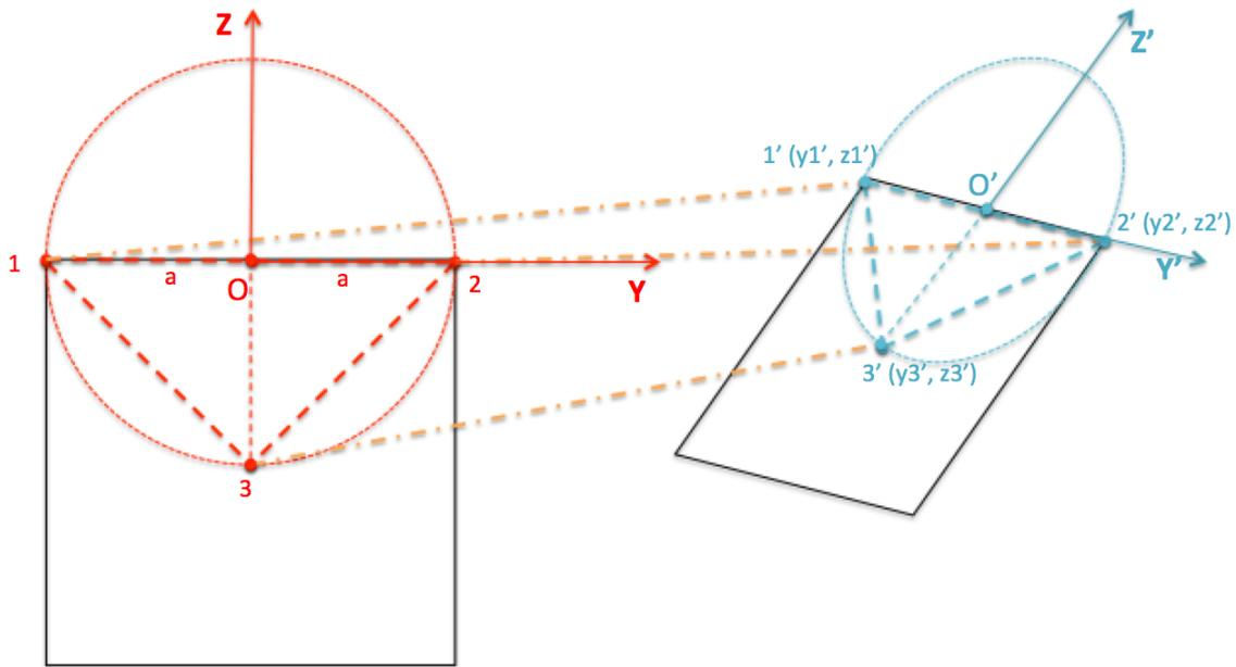
**Standard positions of three corner-cube-reflectors known by the chaser with reference to the chaser's coordinate system assuming the viewing direction is perpendicular with the surface made of OY and OZ which is the one that the corner-cube-reflectors are attached, also the image's plane of the camera**
