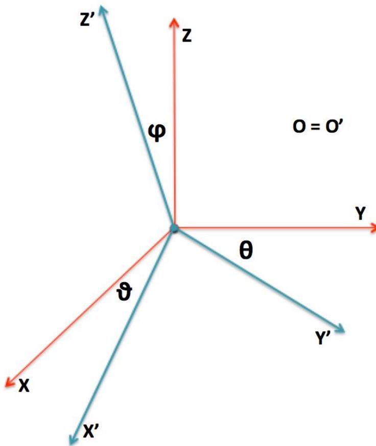
**Figure 41 Demonstrate the three-axes rotation**
