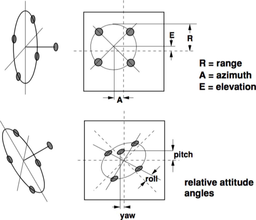
Figure 13 Target pattern for a camera rendezvous sensor<sup>16</sup>
