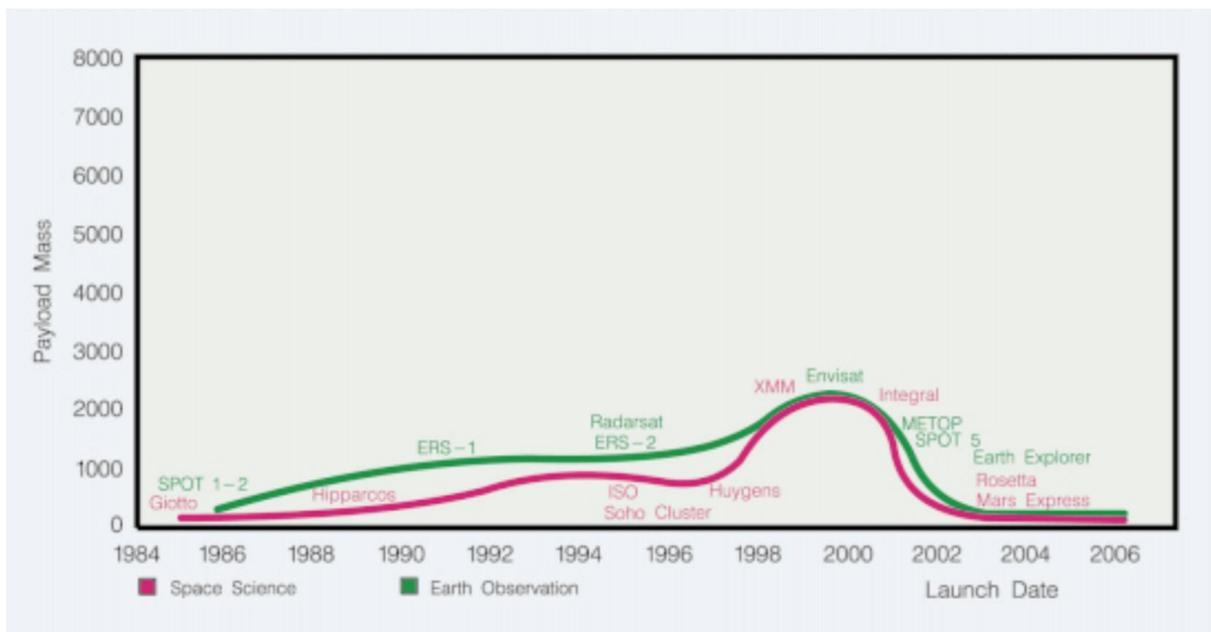
**Figure 4 Payload-mass histories for science and earth observation satellites<sup>6</sup>**
