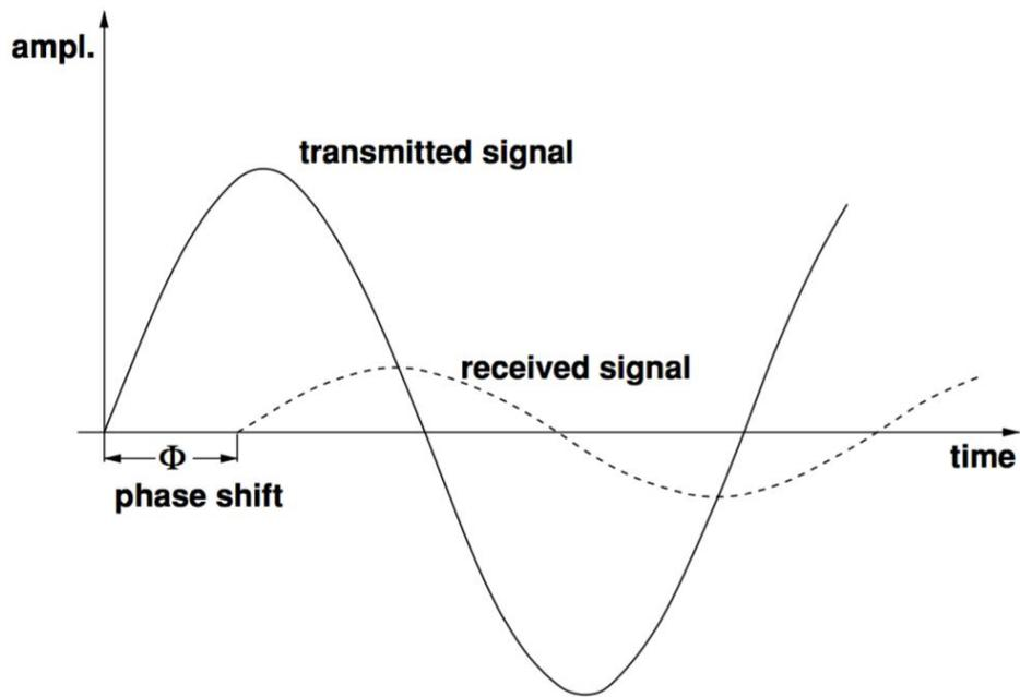
**Figure 6 Functional principle of range measurement via phase shift<sup>9</sup>**
