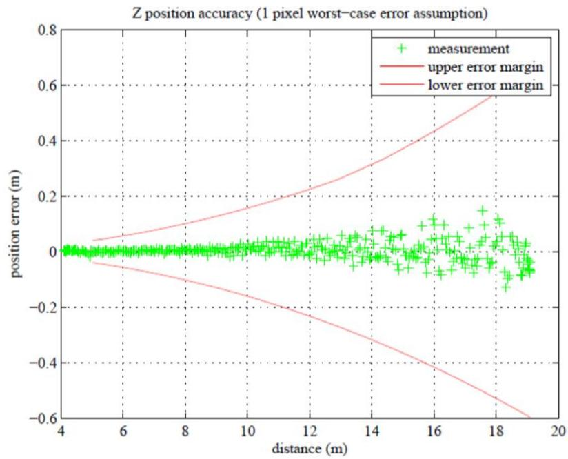
Figure 22 Monocular sensor's range accuracy<sup>27</sup>
