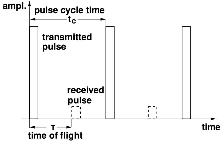
**Figure 5 Functional principle of range measurement via time delay<sup>8</sup>**
