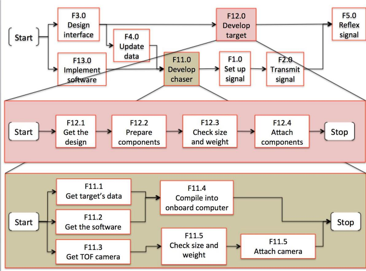
Figure 32 Function break down of F11 and F12
