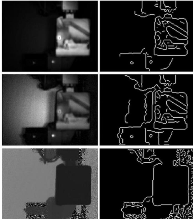
**Figure 17 Canny edge detections using amplitude image (top), intensity image (middle) and depth image (bottom)<sup>21</sup>**
