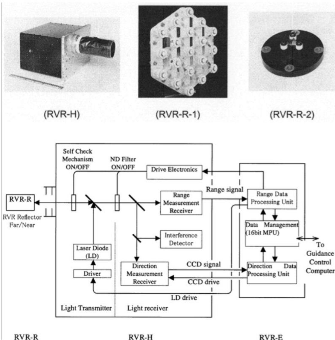
Figure 16 Photo and schematic diagram of the RVR<sup>19</sup>
