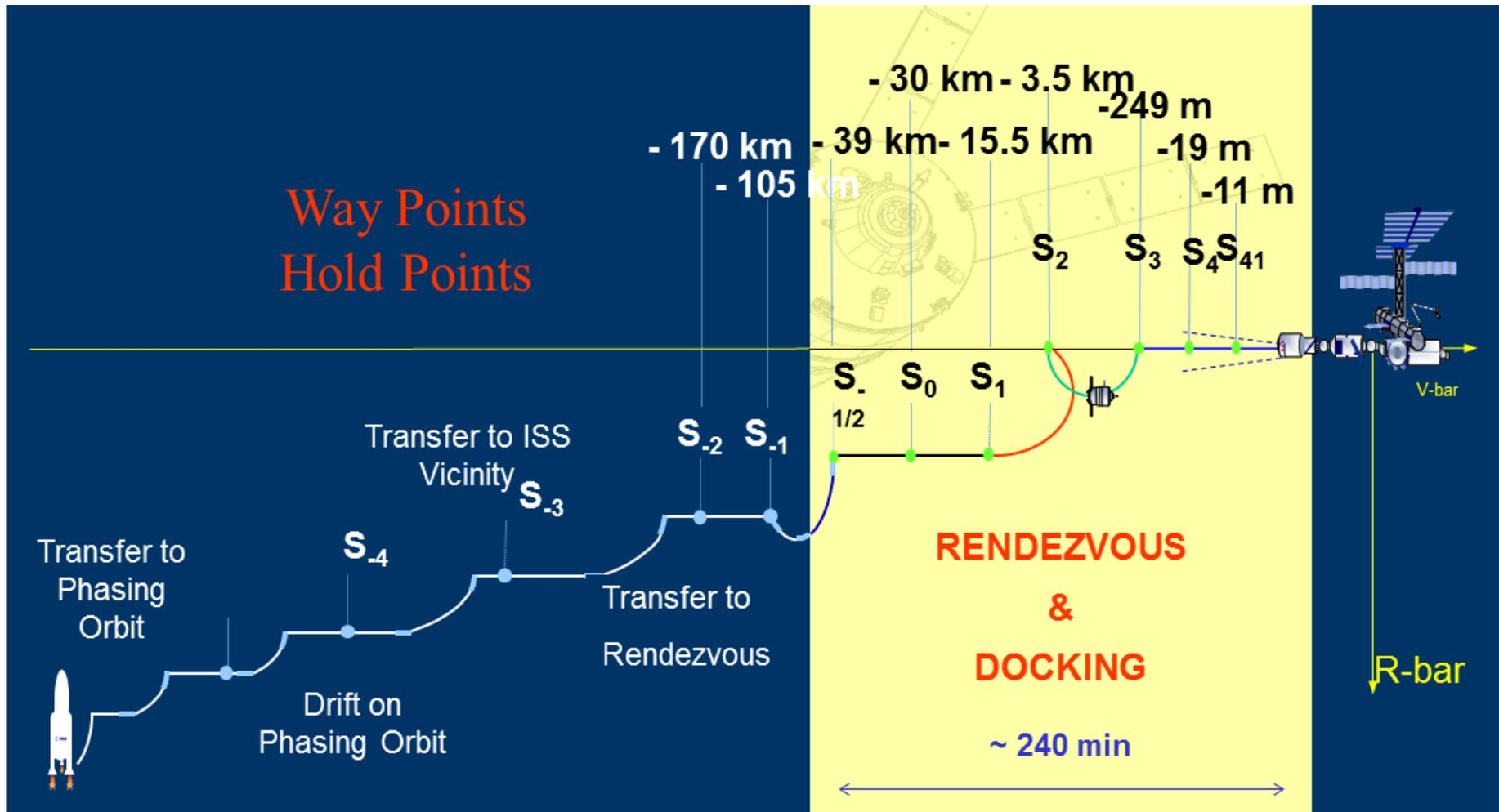
Figure 2 ATV flight profiles in order to supply the ISS<sup>3</sup>
