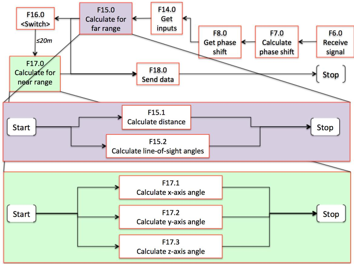
**Figure 33 Function break down of F15 and F12**
