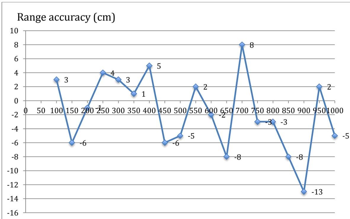
Figure 60 Range determination accuracy
