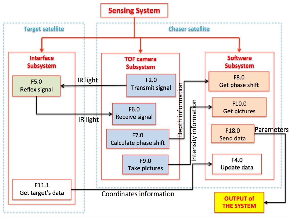
**Figure 50 Architecture diagram of the new sensing system**
