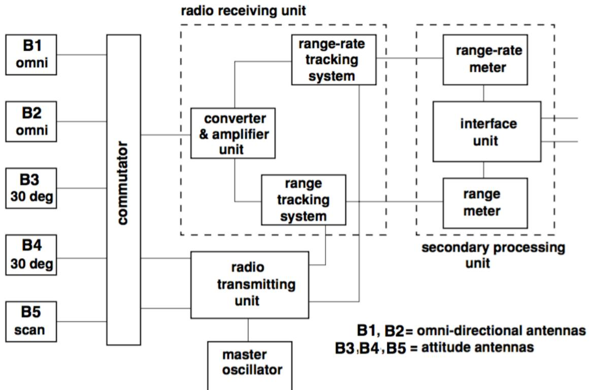
**Figure 9 Functional block diagram of Kurs ‘transponder’ equipment<sup>12</sup>**
