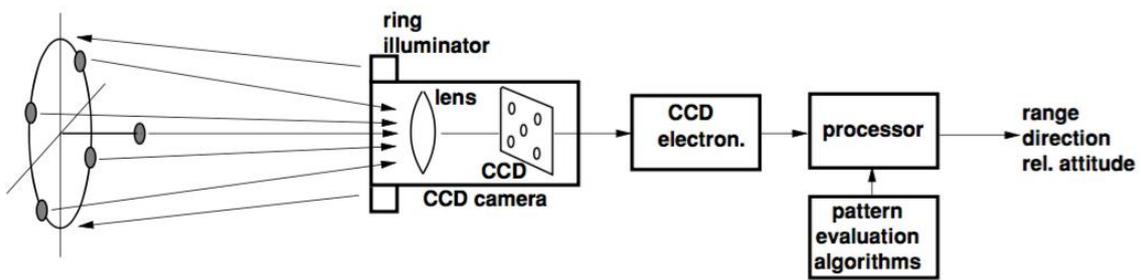
**Figure 12 Functional principle of a camera rendezvous sensor<sup>15</sup>**
