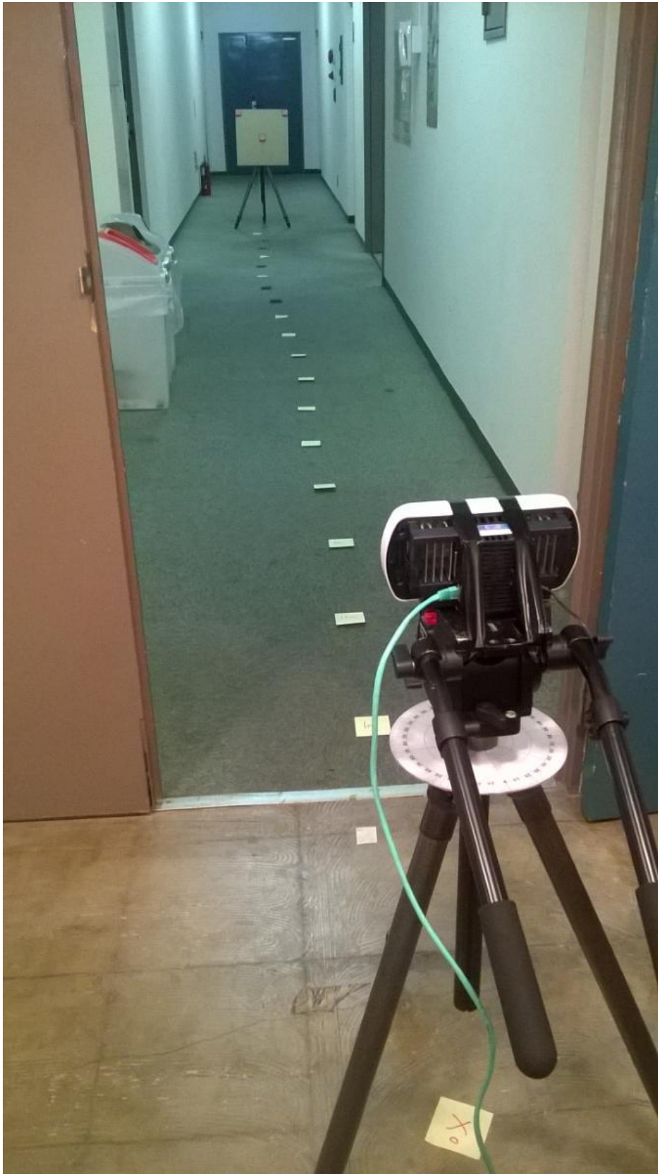
Figure 56 Range determination test
