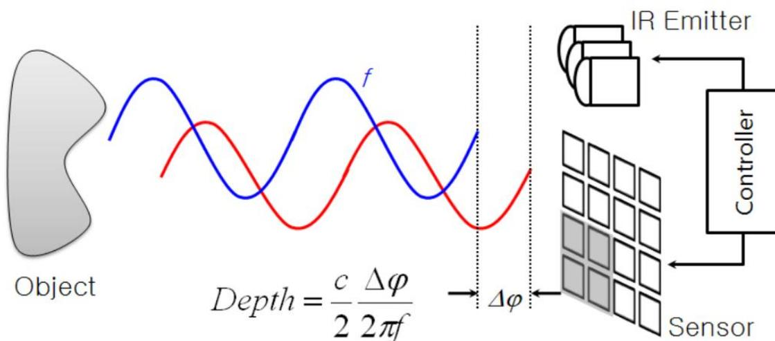
**Figure 25 Principle of TOF depth camera<sup>30</sup>**
