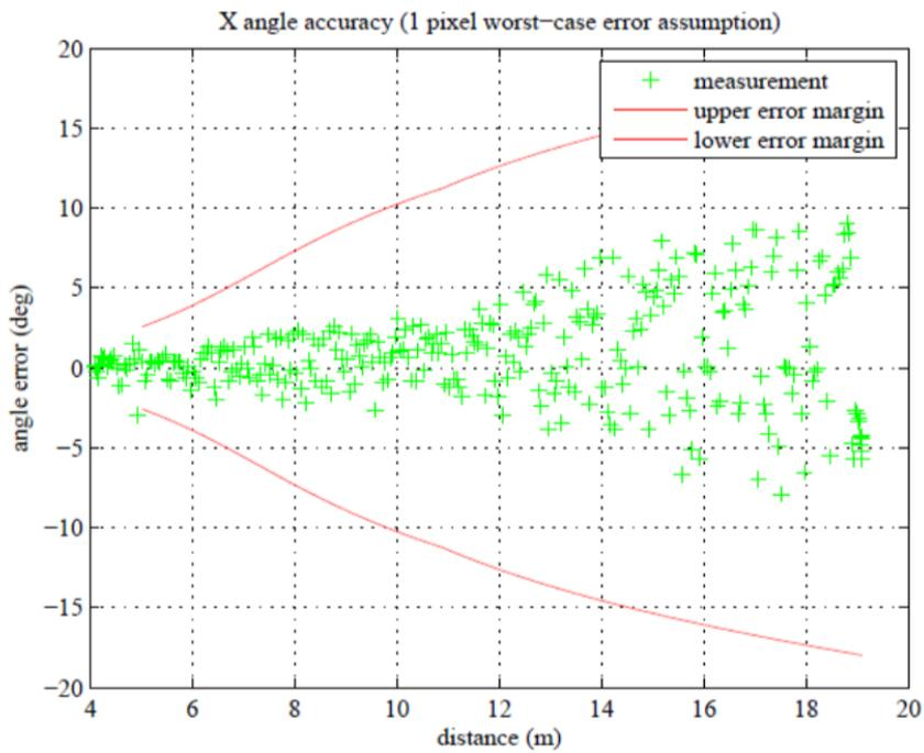
Figure 23 Monocular sensor's angle accuracy<sup>28</sup>
