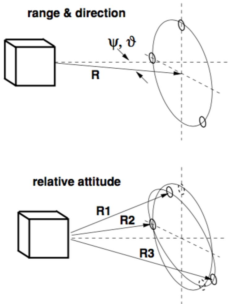
Figure 11 Target pattern for a laser range finder<sup>14</sup>
