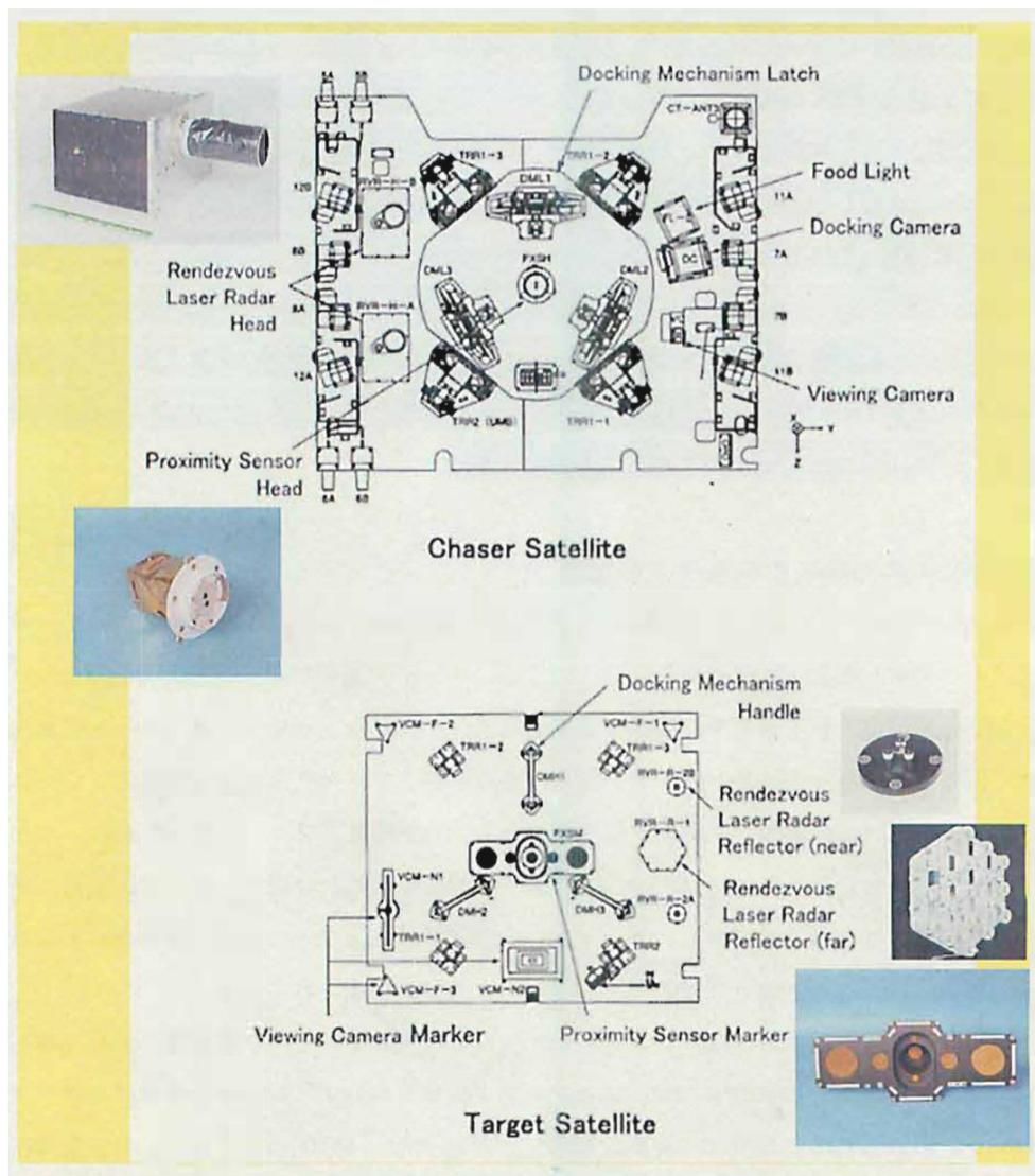
Figure 15 Docking planes of chaser and target satellites<sup>18</sup>
