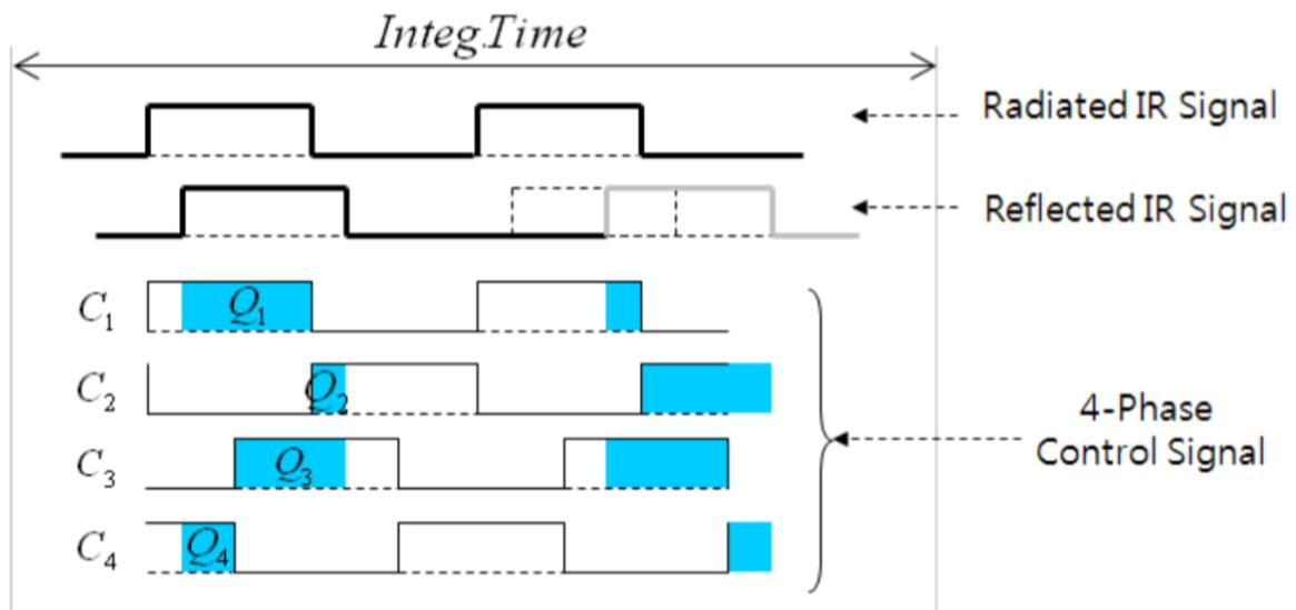
**Figure 26 Phase shift determination<sup>31</sup>**
