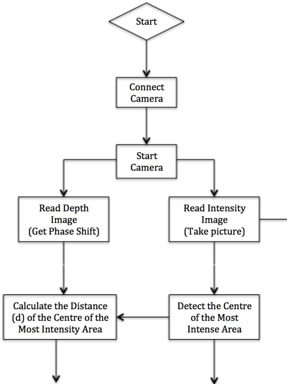
**Figure 47 Software implementation diagram (part 1)**
