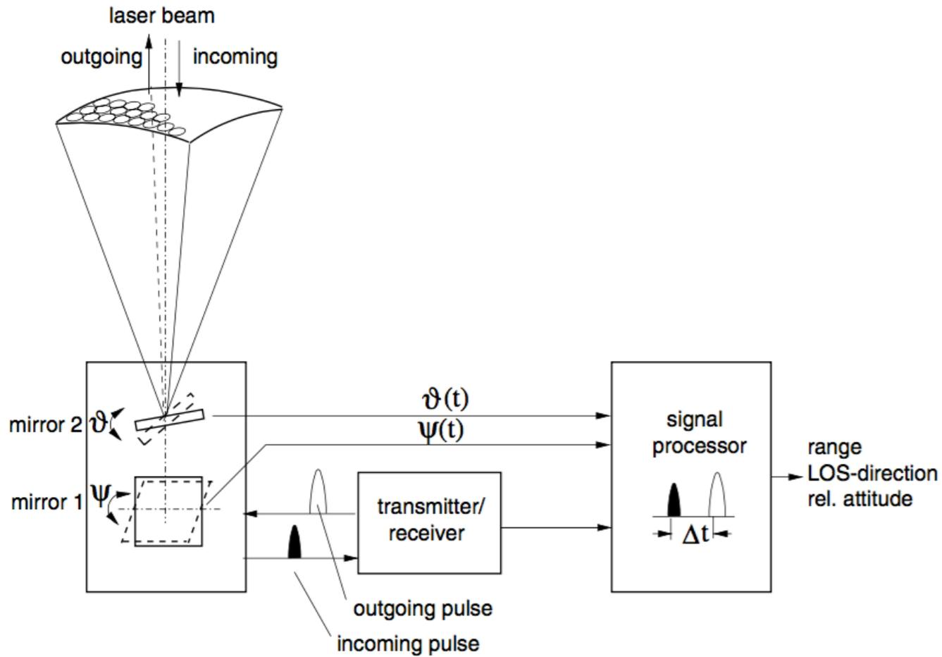
Figure 10 Functional principle of a scanning laser range finder<sup>13</sup>
