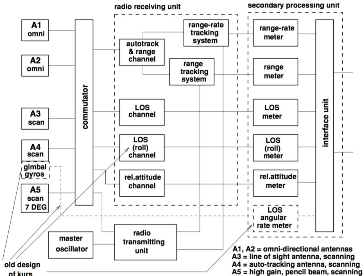
**Figure 8 Functional block diagram of Kurs ‘interrogator’ equipment<sup>11</sup>**
