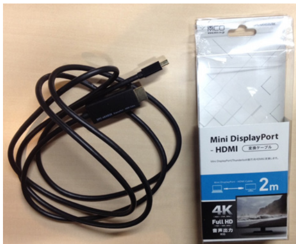
図 4-7 Mini Display Port (Thunderbolt 端子)-HDMI 4K:3840×2160 30Hz Full HD:1920×1080 60Hz
