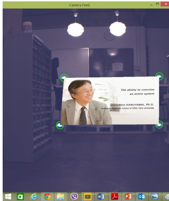
Figure 33: Finally virtual information is superimposed over real environment at the points computed earlier
