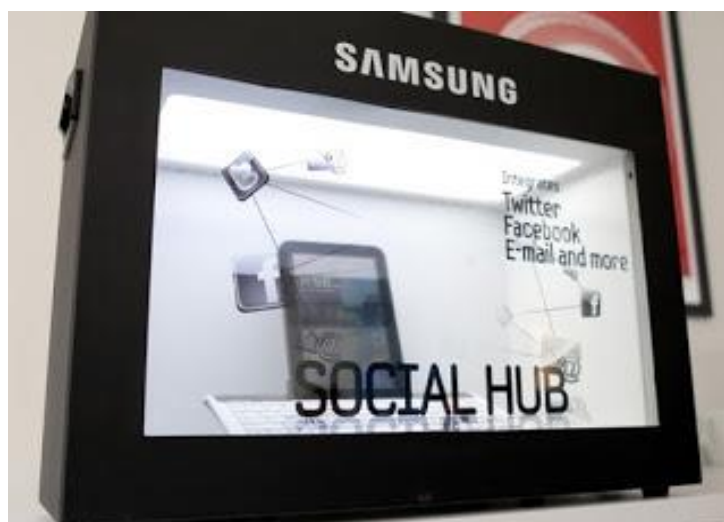
Fig.2-1: Image of Transparent LCD
