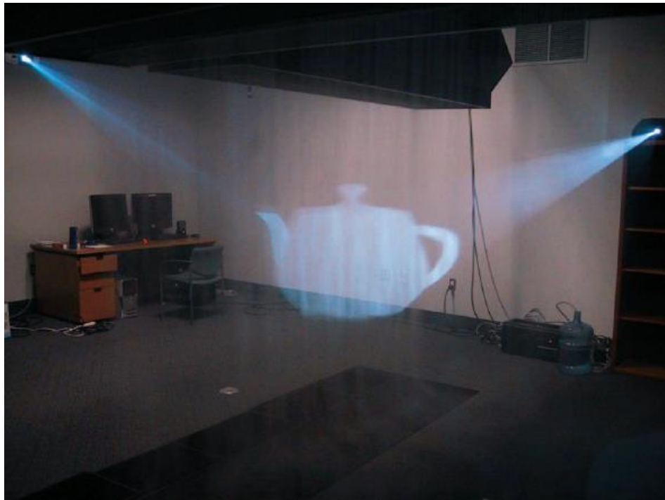
Fig.2-10: Immaterial DFD display using two fog screens
