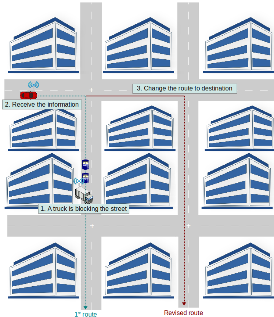
Figure II.19: Obstacle warning example
