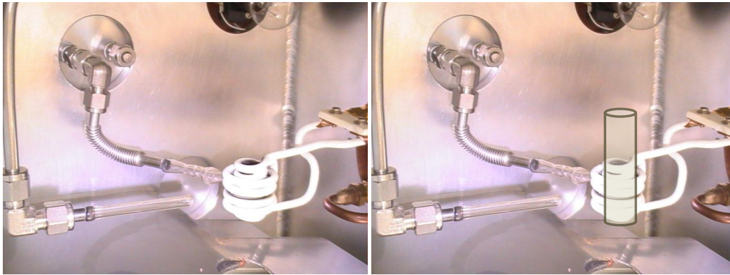
Figure 3.3: Difference of oxygen partial pressure control method on PFLEX experiment. The current model and suggested model.
