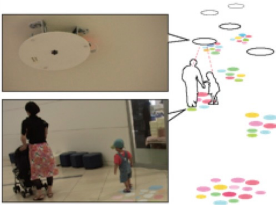
Figure 3.16: Sensor system of Sound Entrance
