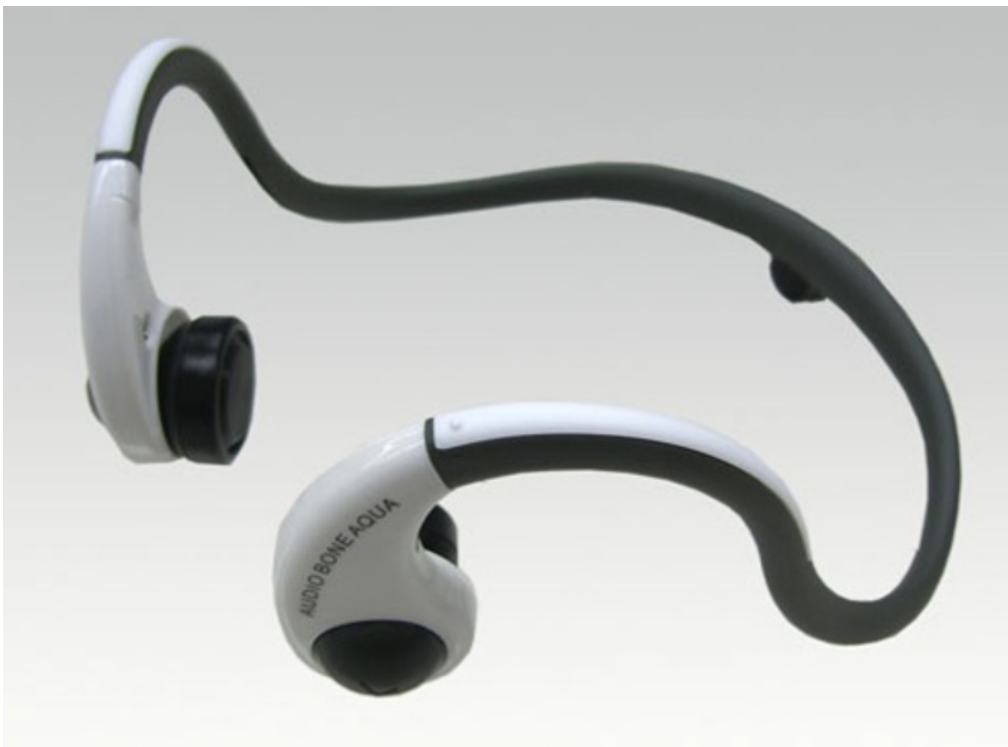
Figure 4.7: Bone conductive headphones that were used by users to address safety issues and prevent the Navinko application from blocking users hearing of their surrounding. Photo by author.
