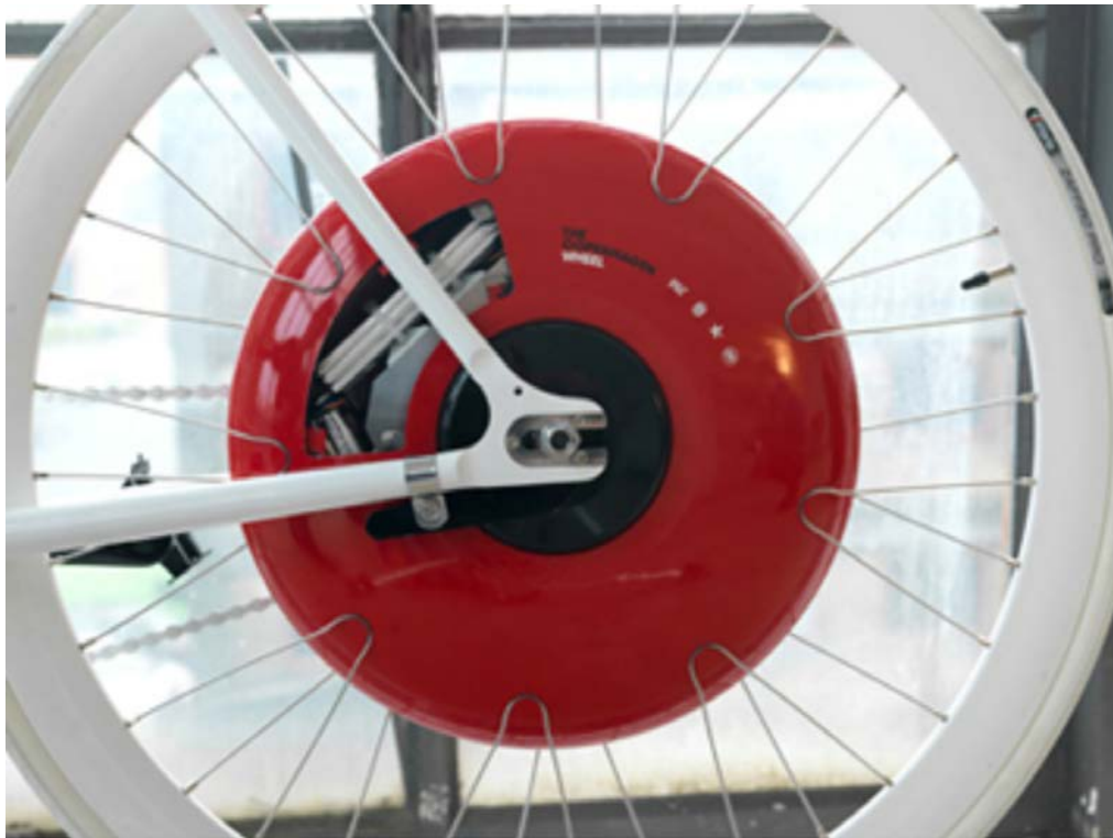
Figure 2.13: Copenhagen Wheel. Sensor network and riding support. Source: Copenhagen Wheel.
