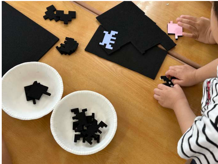
Figure 4.8 Conductive sponge precut by laser cutter (1).
