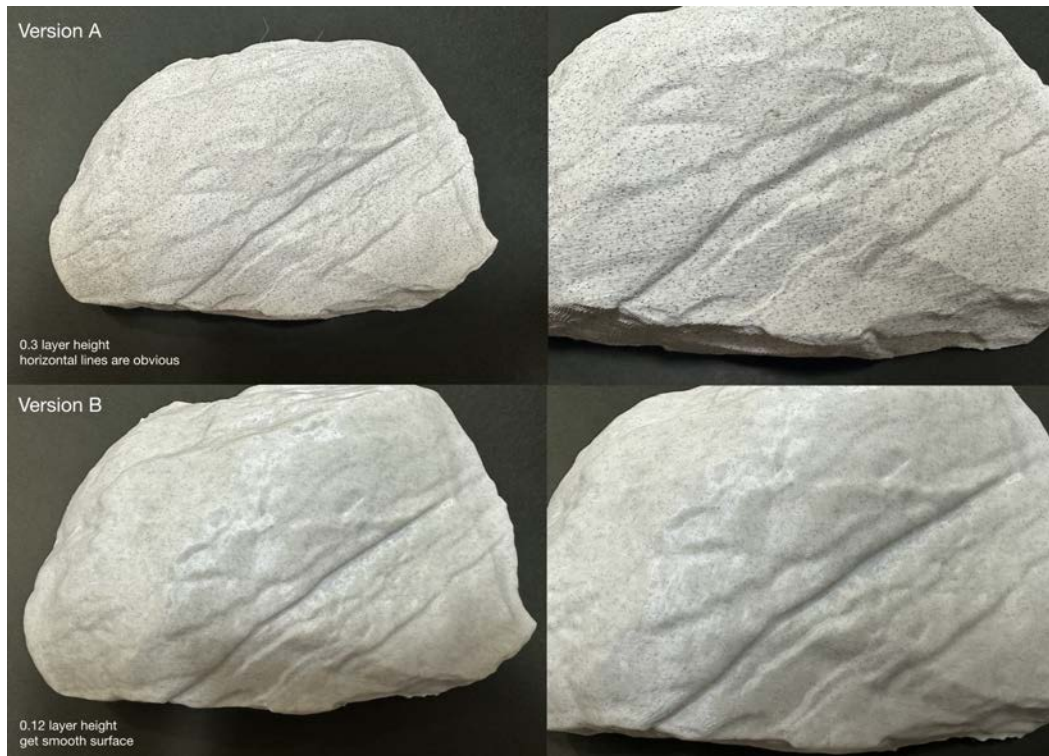
Figure 4.3 Two Versions of 3D-Printed Shell
