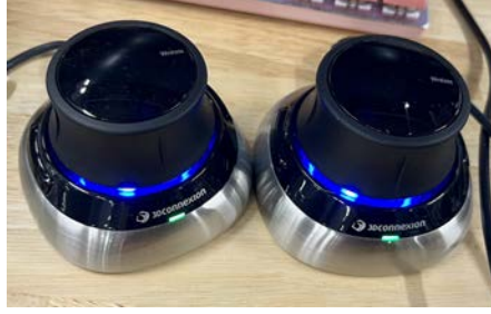
Figure A.3 The SpaceMouse by 3Dconnexion, a 3D joystick designed for CAD software.
