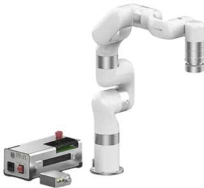
Figure 3.7 xArm 7, a 6 degree of freedom robotic arm by uFactory.
