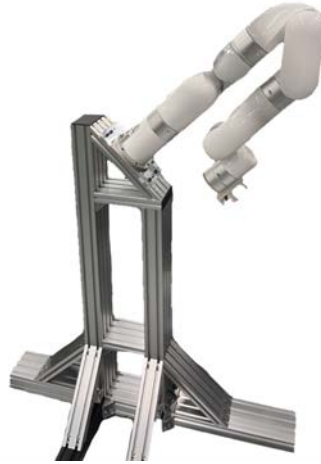
Figure 3.13 The xArm is mounted on a custom aluminum frame stand which tilts the arm forward 45 degrees on the x-axis.
