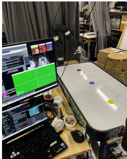
Figure A.2 Prototype of Asura using color blob tracking for 3 pucks.
