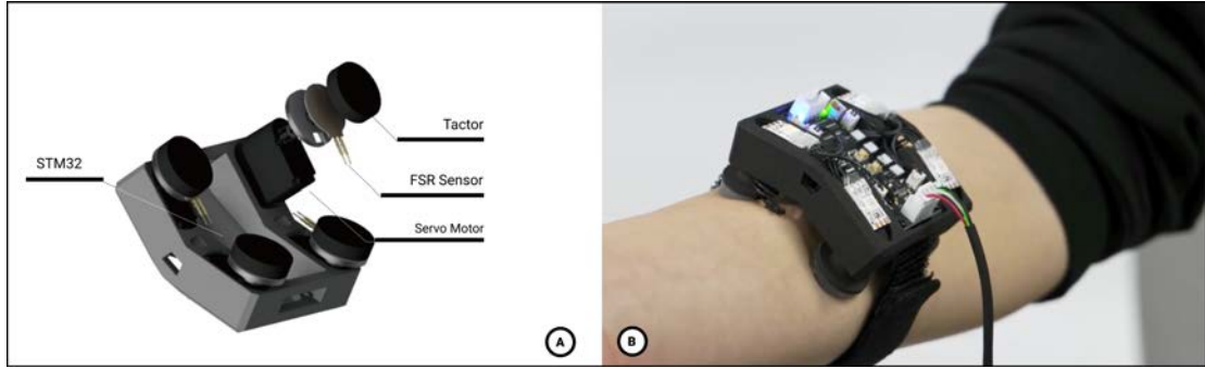
Figure 3.7 (A) Components of the hardware (B)Wearing image
