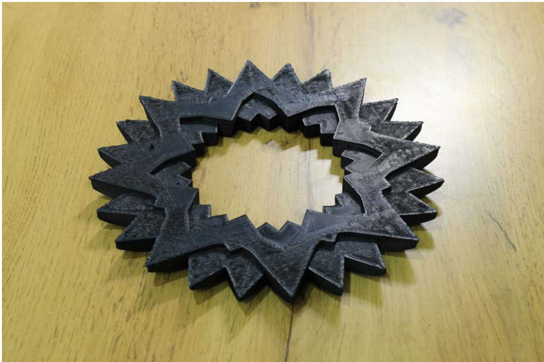
Figure 3.3 Initial physical prototype (first iteration) using black filament. Despite achieving the desired intricate geometry, this prototype lacked LED integration and sufficient translucency, indicating the need for iterative refinement.
