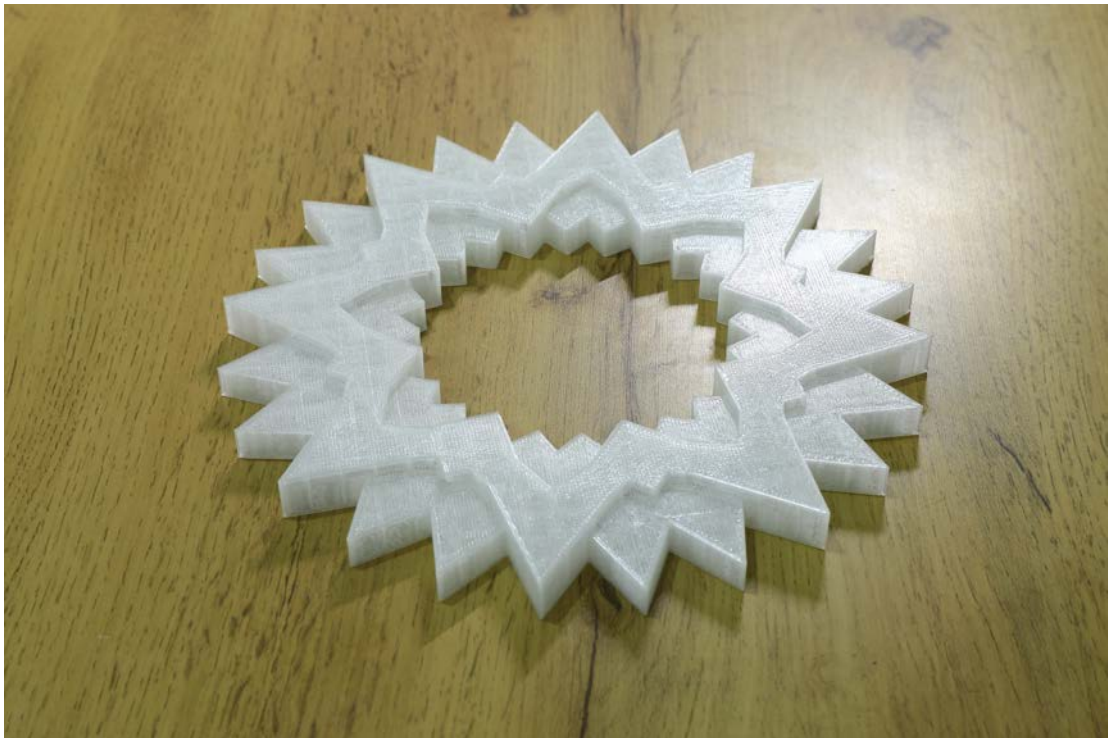
Figure 3.4 Another first-iteration prototype employing a fine-grade, semi-transparent filament. Though LEDs were not yet integrated, this material choice suggested improved future light diffusion potential.
