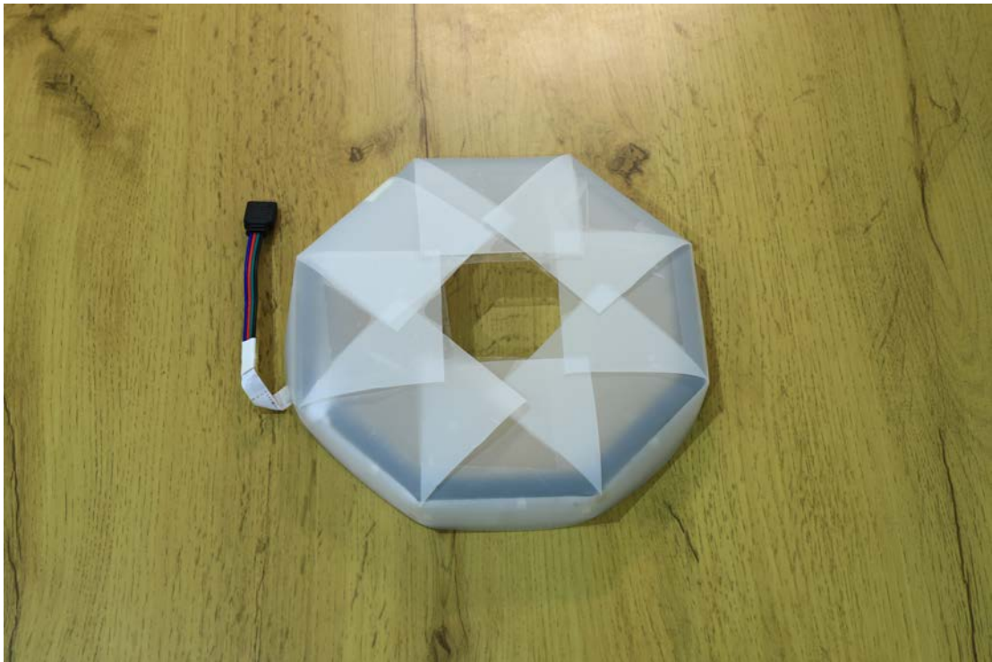
Figure 3.7 Second iteration prototype before LED activation. The absence of glare and careful planning for LED placement allowed the device to be prepped for diffusive layers.
