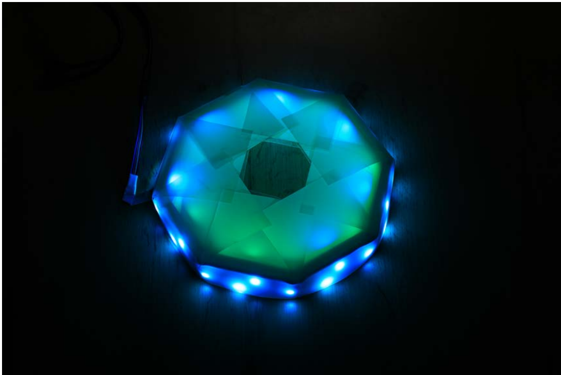
Figure 3.8 Second iteration prototype with the meticulously applied diffusive plastic film. This layer softened the LED light, resulting in gentler, more interpretable visual cues that closely matched intended emotional representations.
