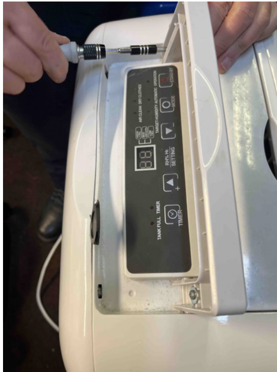
Figure 3.17 Finding the location of the screws is problematic
