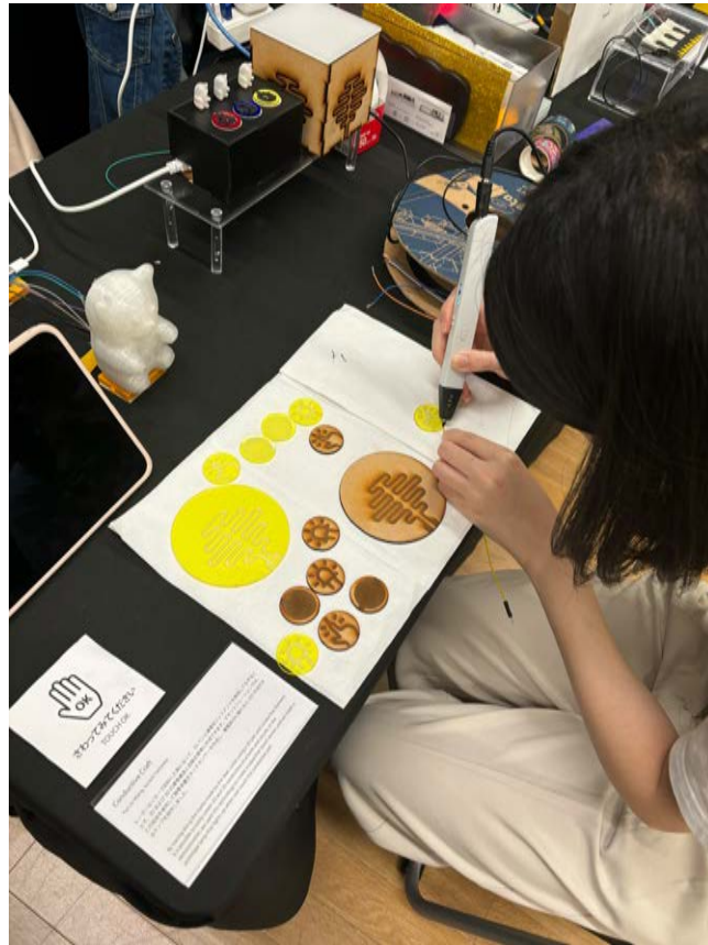
Figure 5.1 The participant is using the 3D pen and conductive filament to trace along the engraved circuit pattern.
