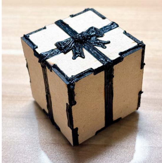
Figure 4.21 A 3D structure is form with 3D pen and conductive filament.
