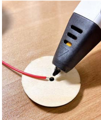
Figure 4.14 The 2.5mm hole serves as an interface for easy wire connections using a 3D pen after completing the circuit samples.
