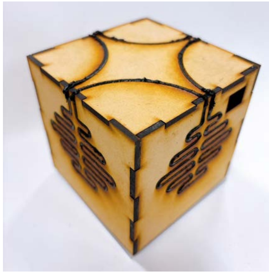
Figure 4.7 The bottom face of the box, showing how the interactive circuits on each side are connected together to form a complete circuit.
