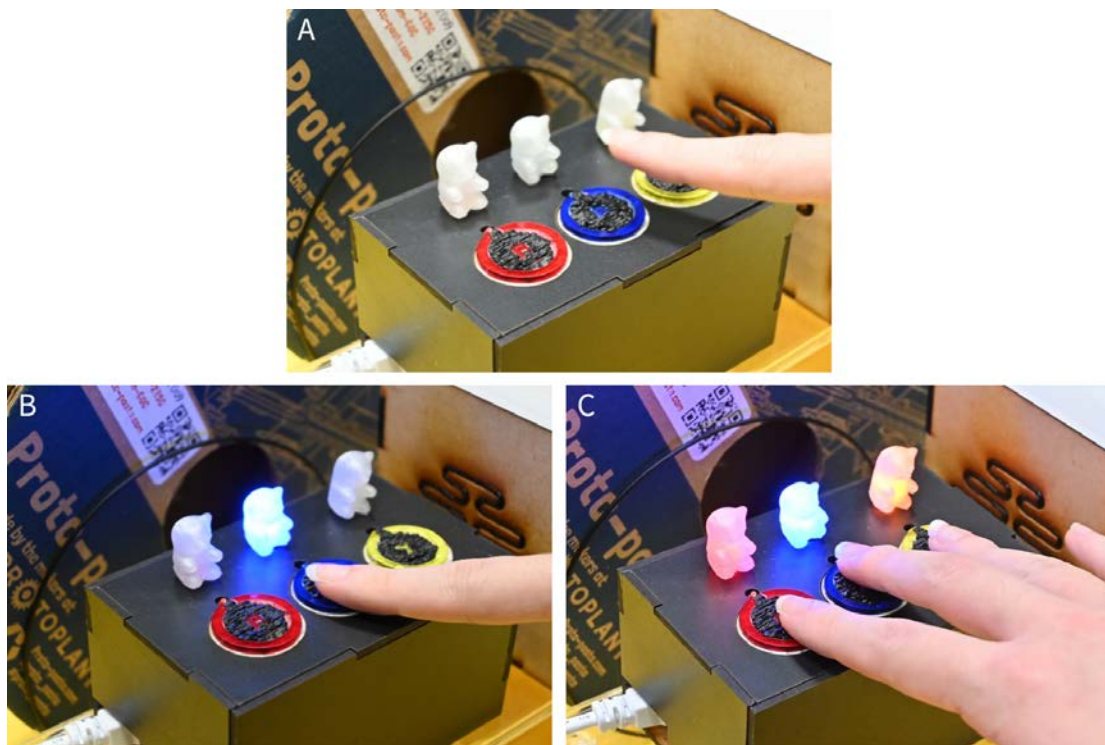
Figure 4.1 Interactive device with simple touch sensor buttons. A: When no button is touched. B: When a button is touched, the corresponding LED lights up. C: When multiple buttons are touched simultaneously.
