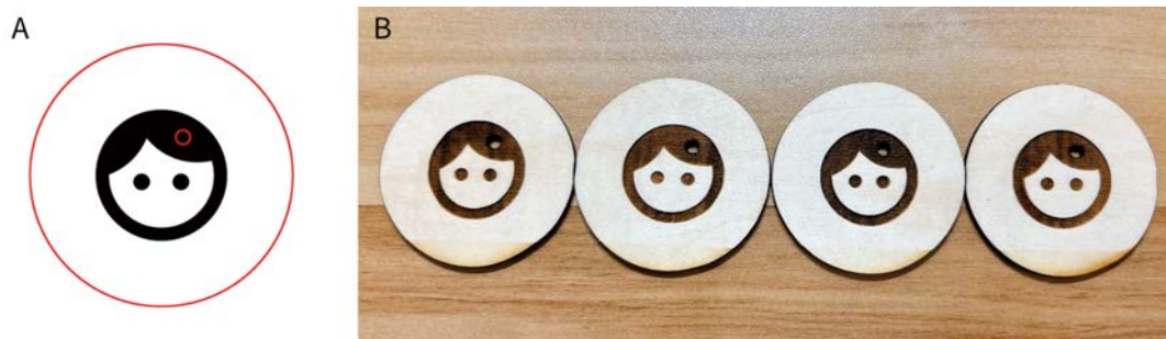
Figure 4.17 Design of Prototype III Part 3. A: Laser Cutting Design.(red lines for cutting, black areas for engraving). B: Samples after laser cutting.
