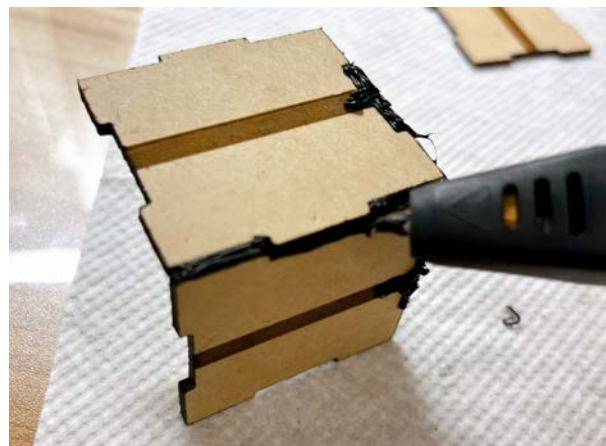
Figure 4.20 Connecting each face with 3D pen and conductive filament.
