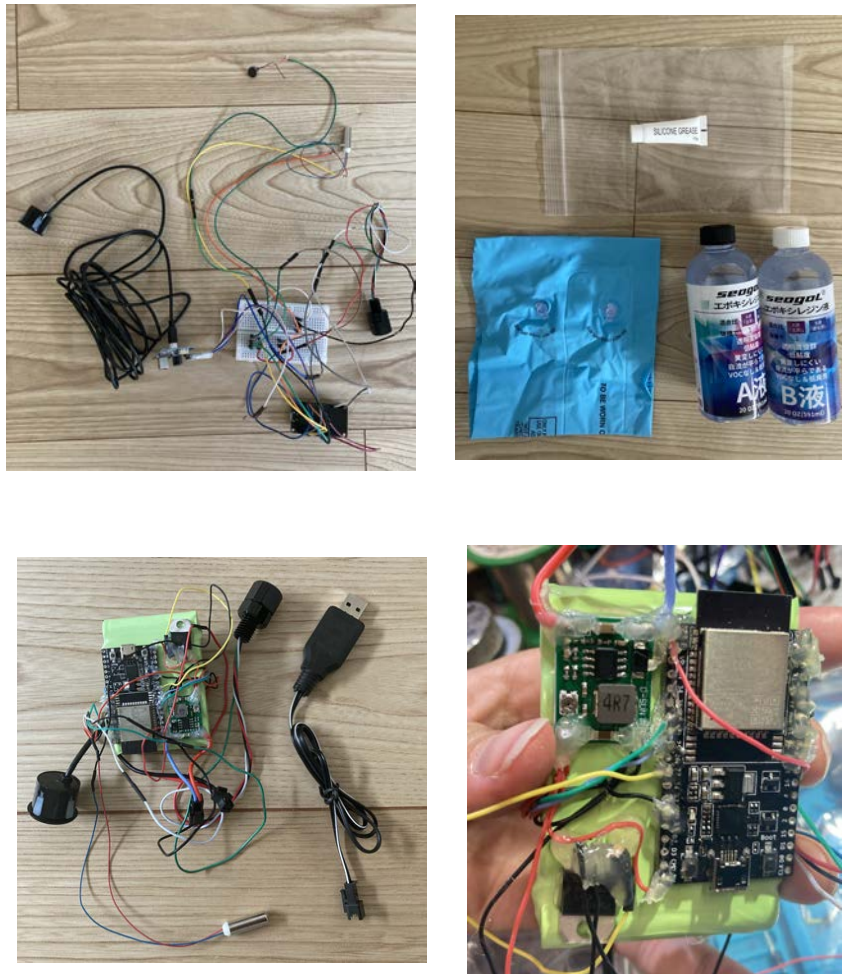
Figure 3.9: Waterproofing tools and waterproofing the sonar-haptic unit
