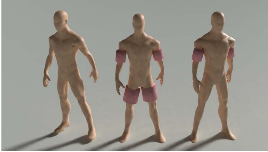
Figure 4.3: Three haptic-sonar unit locations from the left: (a) none, (b) four locations, and (c) two locations.
