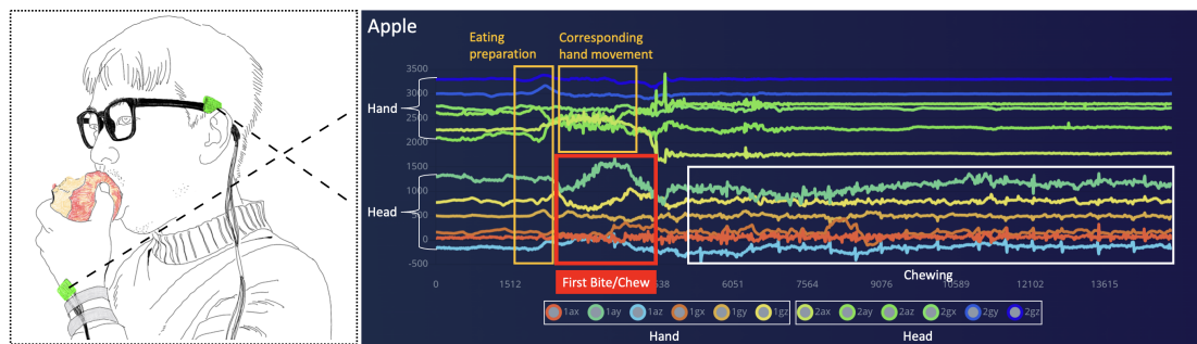
Figure 3.2 When a participant consumes an apple, we collect 12 axes of IMU data related to their eating movements, as shown in the Waveform plot on the right side. The length of the red rectangle represents the portion we define as the first bite/chew, while the thin yellow rectangle indicates the preparation of hand and head movements before eating.
