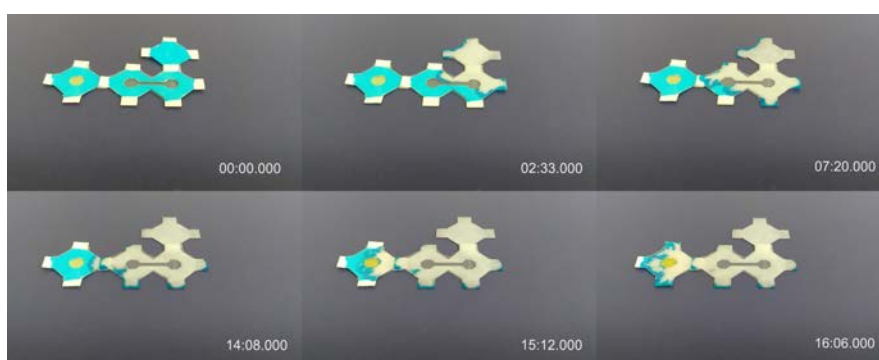
Figure 4.4 Liquid Flow in a Device with Time for Narrow Channels
