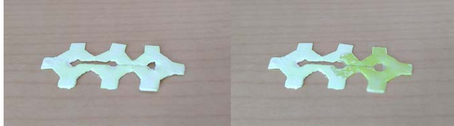
Figure 3.7 Liquid Flow When Hydrochromic Ink is Used
