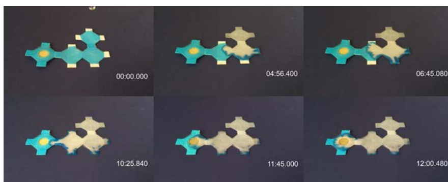
Figure 4.5 Liquid Flow in a Device with Time for Wide Channel
