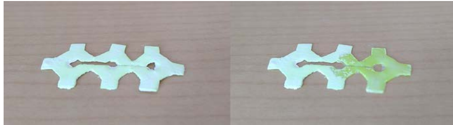
Figure 3.7 Liquid Flow When Hydrochromic Ink is Used
