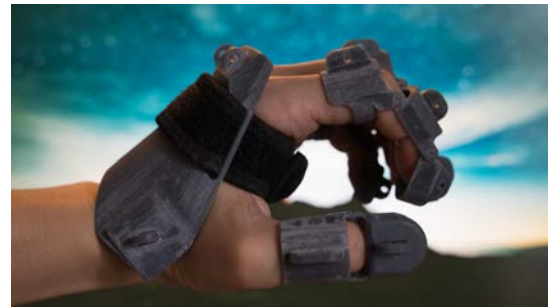
Figure 3.83 New exoskeleton assembly - closed position
