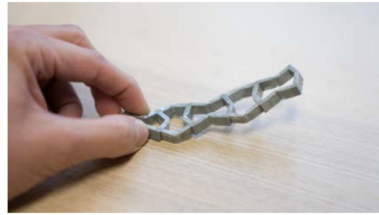
Figure 3.40 The 3D printed structure deformed and bend when compression is applied on the first block
