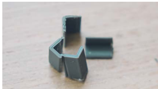
Figure 3.38 The block was broken when compression is applied due to the lack of malleability of the material
