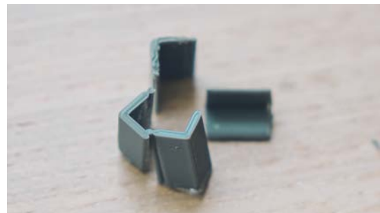
Figure 3.38 The block was broken when compression is applied due to the lack of malleability of the material
