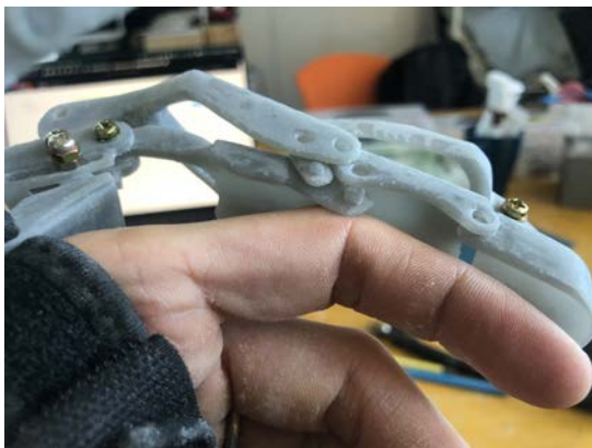
Figure 3.107 Diameter of exoskeleton too small
