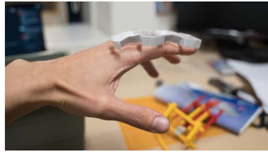
Figure 3.34 The paper prototype sitting on the back of the index finger for size fitting of the exoskeleton
