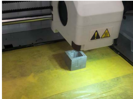
Figure 3.36 A compliant four-bar linkage block being printed
