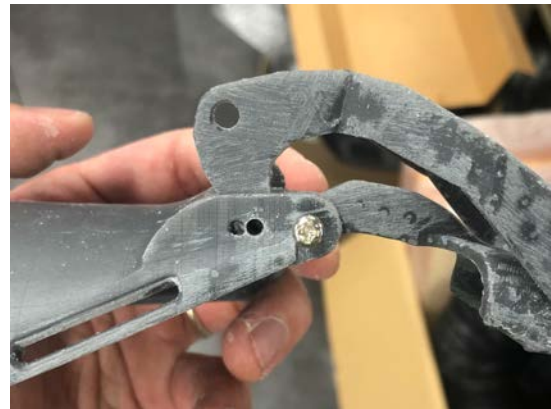
Figure 3.118 Hole drilled on palm component
