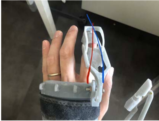
Figure 3.109 Misalignment between finger and exoskeleton
