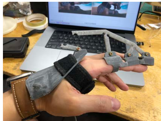
Figure 3.89 Compliant backbone broken
