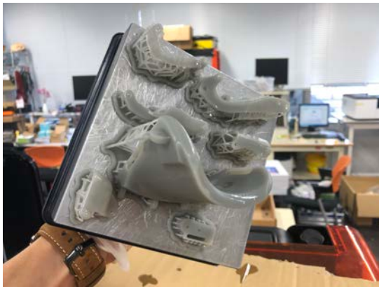
Figure 3.98 3D printed components on the build platform
