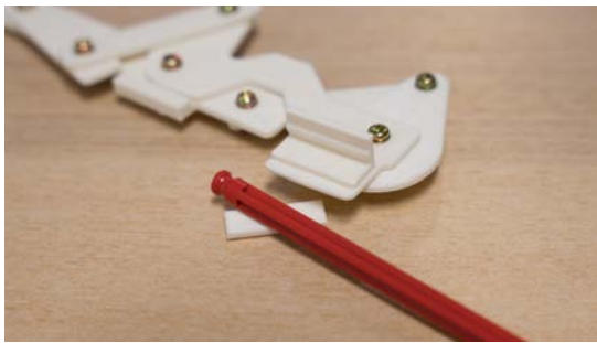
Figure 3.50 A broken K'nex joint
