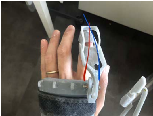
Figure 3.109 Misalignment between finger and exoskeleton
