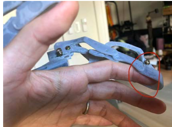
Figure 3.108 Finger cannot slide beyond the cap
