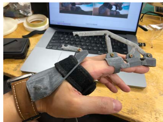
Figure 3.89 Compliant backbone broken
