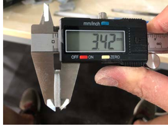
Figure 3.101 Inaccurate dimension of printed component
