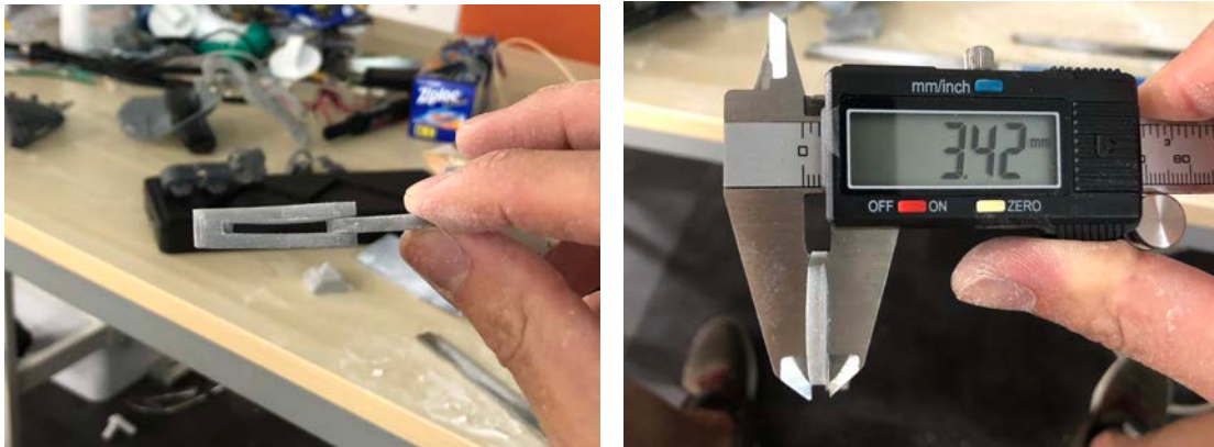
Figure 3.100 Bulge in printed component
