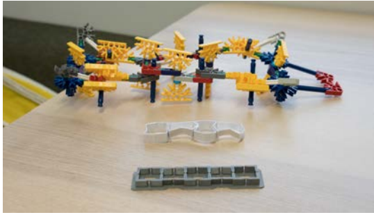
Figure 3.39 Top: K'nex prototype; Middle: Paper prototype; 3D printed prototype
