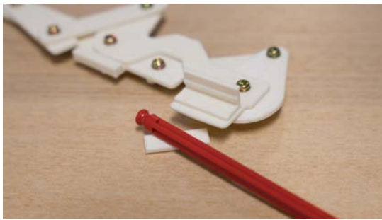
Figure 3.50 A broken K'nex joint
