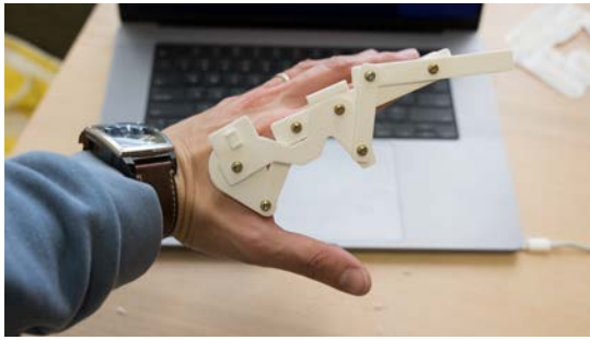
Figure 3.48 New finger mechanism printed and assembled
