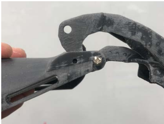
Figure 3.117 Misalignment between finger and palm
