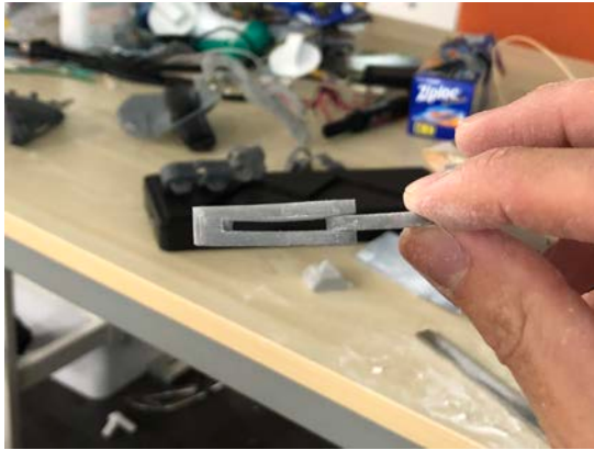
Figure 3.100 Bulge in printed component
