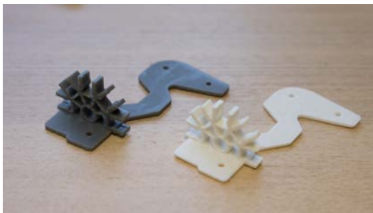
Figure 3.52 Left: SLA Printed Prototype Right: FDM Printed Prototype
