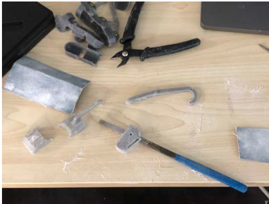
Figure 3.102 Sanding of individual components
