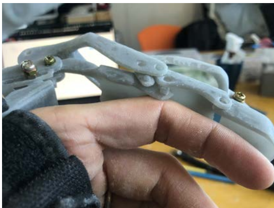
Figure 3.107 Diameter of exoskeleton too small
