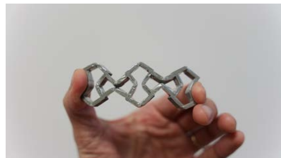
Figure 3.42 The structure under complete deformation
