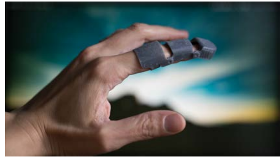
Figure 3.77 3D printed finger prototype fit test
