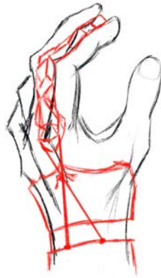
Figure 3.25 Early sketch of an exoskeleton device: the red sketch shows how the device attaches to the user's hand
