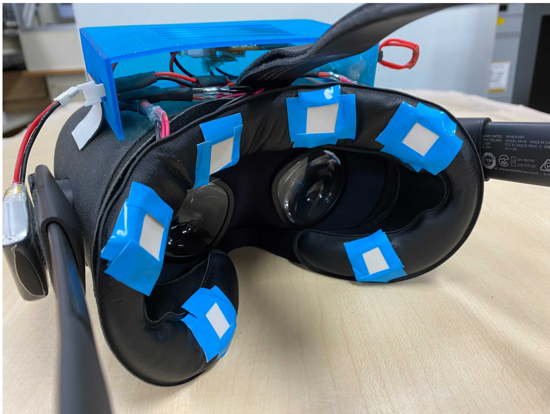
Figure 4.1 The prototype of mobile head-mounted display with thermal feedback
