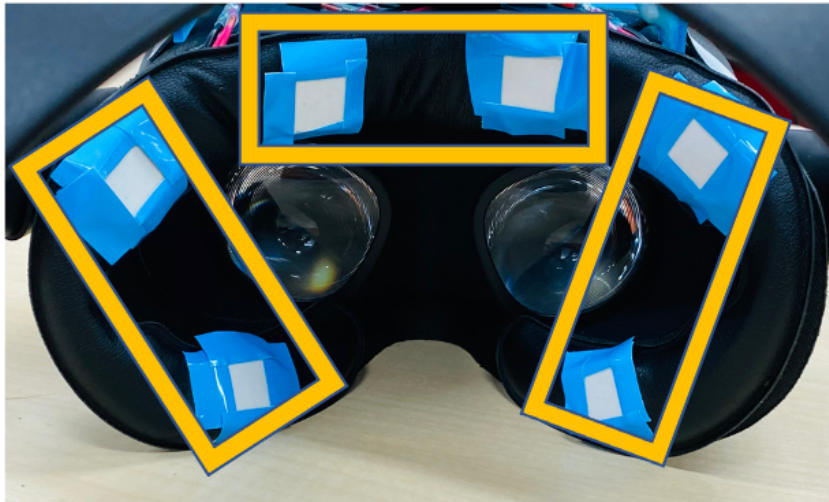
Figure 4.14 6 Peltier elements are split into 3 channels
