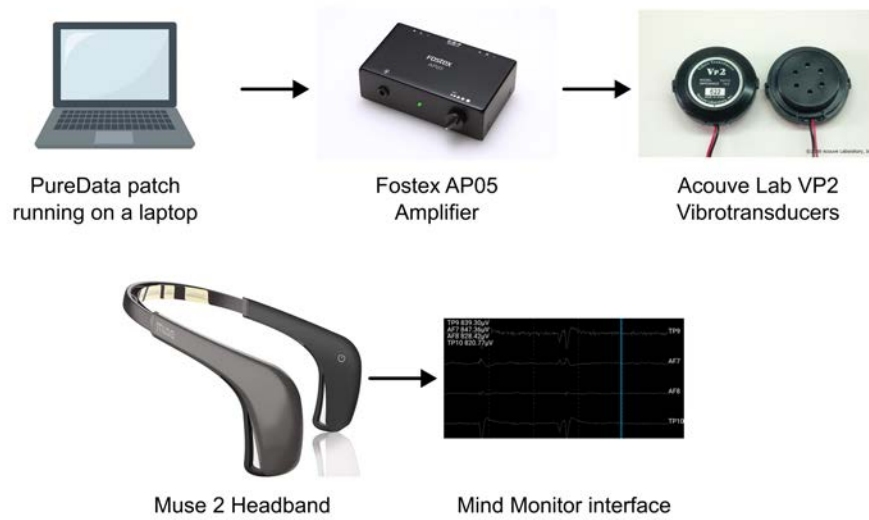
Figure 3.3 The first prototype and the neurofeedback loop 1
