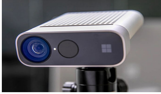
Figure 2.5: Microsoft Azure Kinect: RGB-D Camera
