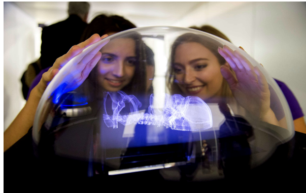
Figure 2.11: Voxon Photonics Volumetric Display
