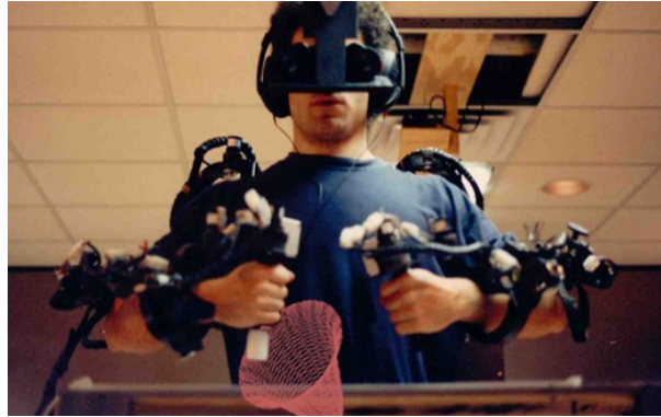
Figure 2.1: Virtual Fixtures Kinaesthetic Exoskeleton (1992)
