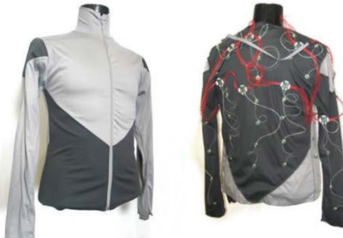
Figure 2.5 A body-conforming tactile jacket to enrich movie viewing
