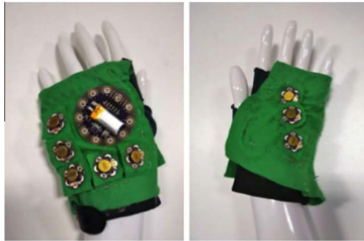
Figure 2.4 Mood Glove: A haptic wearable prototype system [2]
