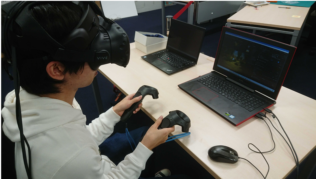
Figure 4.11 Subjects wear an VIVE head-set with the fNIRS device which connected computer over the bluetooth
