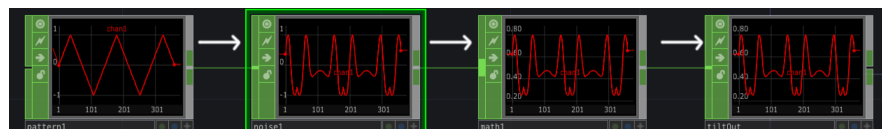
Figure 3.15 Touch Designer nodes for creating and modifying a triangle wave, making resulted movement indirect.
