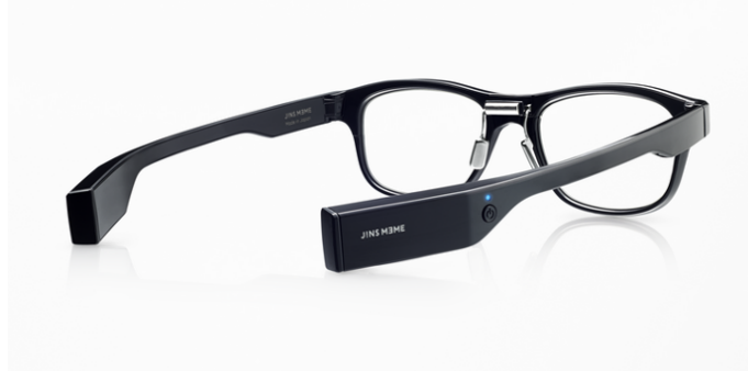
Figure 2.10 EOG-enabled smart eyewear, J!NS MEME
