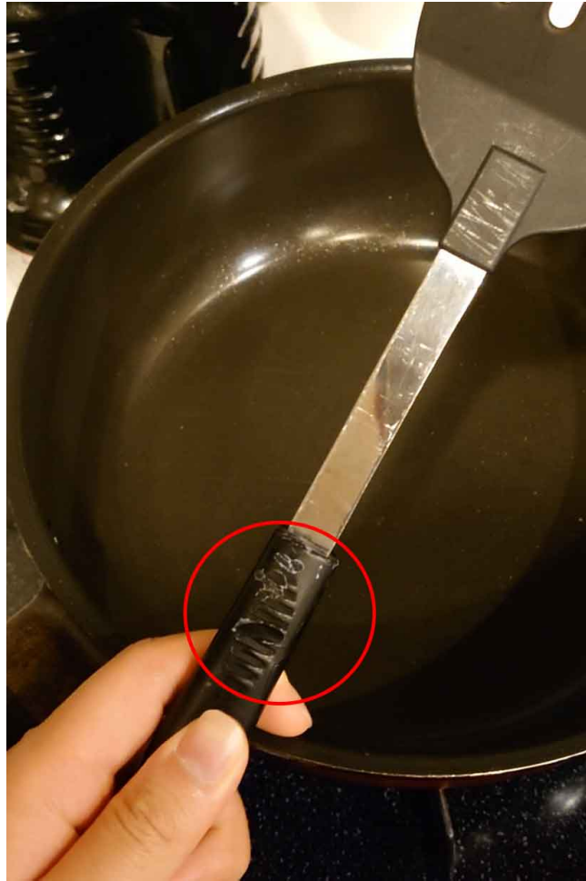
Figure 4.5 Heat Damage in A Spatula
