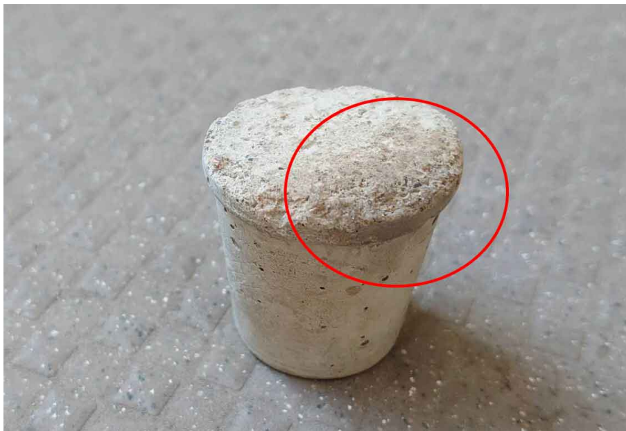
Figure 4.2 Color of Surface Turned Brown at 600 degrees
