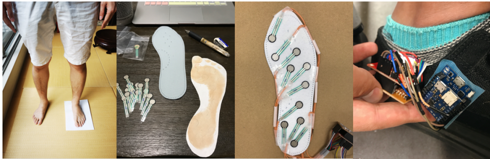
Figure 4.8 Design and implementation process of the first prototype mainly on the inner side of the feet.
