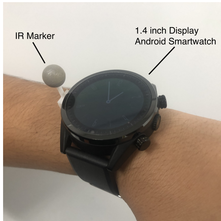
Figure 4.3 Smart watch prototype equipped with IR Marker
