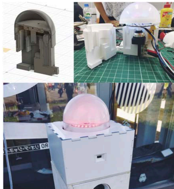
Figure 4.21 Modeling and Fabrication - Interactive Button
