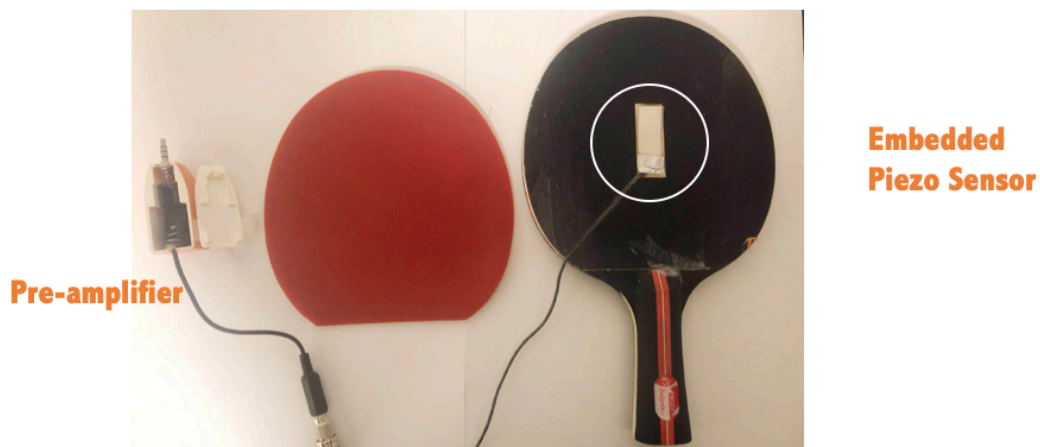
Figure 3.9 Redesigned racket with embedded sensor
