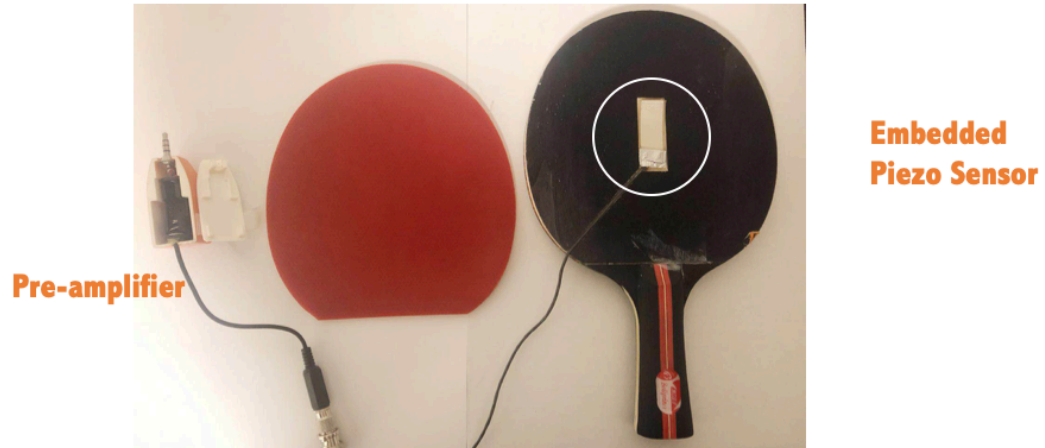
Figure 3.9 Redesigned racket with embedded sensor
