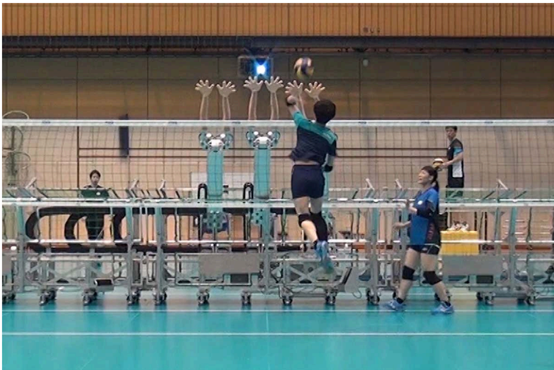
Figure 2.10 A block machine for volleyball attack training
