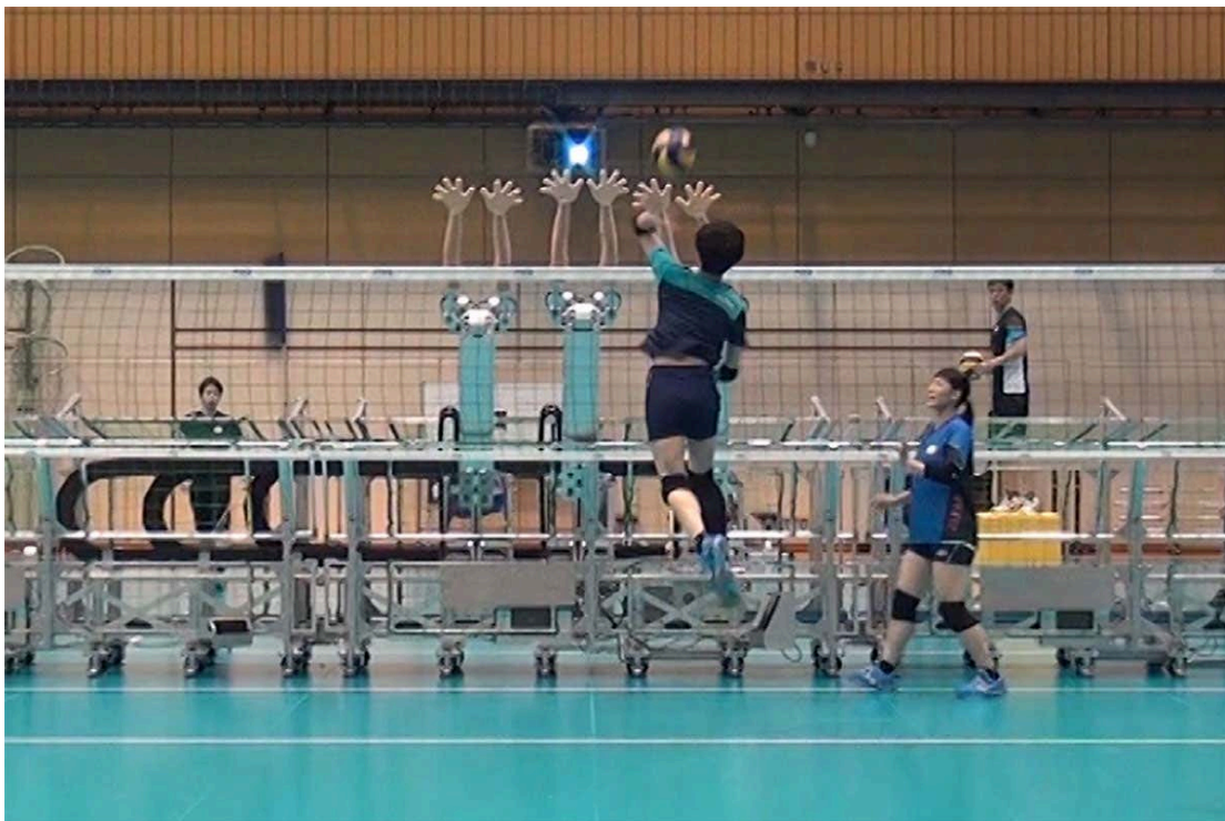
Figure 2.10 A block machine for volleyball attack training
