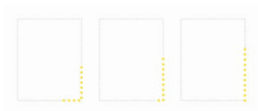
Figure 4.3 running lighting pattern
