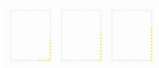
Figure 4.9 running lighting pattern
