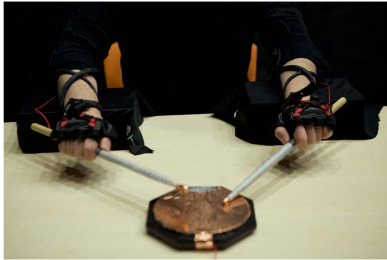
Figure 3.8 PGM is attached with both arm and it actuates the arm for drumming.
