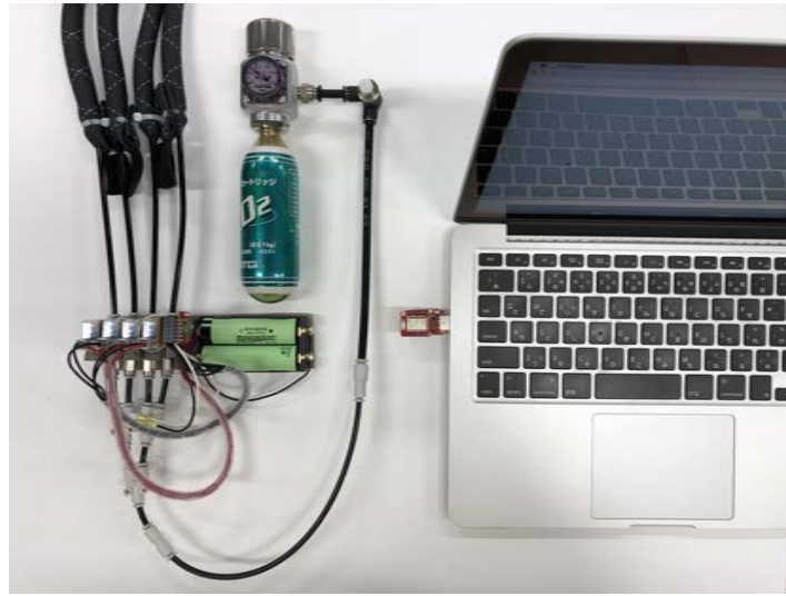
Figure 3.2 The device consists of artificial muscle, solenoid battery, BLE nano v2, gas cylinder. This allows us our prototype based on a laptop computer with a USB Bluetooth 4.2 dongle.
