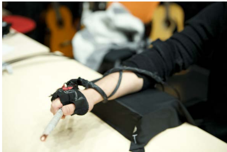
Figure 3.7 The each arm is wrap up with two PGM to actuate hand for pronation and supination.
