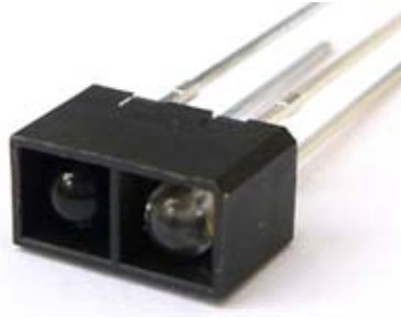
Figure 3.3 Photograph of proximity sensor LBR-127HLD
