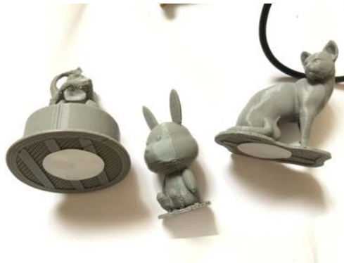
Figure 4.4 Character with RFID tag
