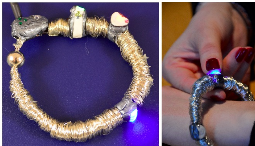
Figure 2.14: Prototype of the Tangible Apps Bracelet. Each element is made up by plastic material, and they release lights under mounts of LEDs. These LEDs are moulded into various aesthetic styles, glued on the buttons, painted and decorated with propylene. The author team wound the silver thread around the copper wire to form a plasticity bracelet to make the appearance more beautiful. Right: the user realizes input by pushing the element. [6]
