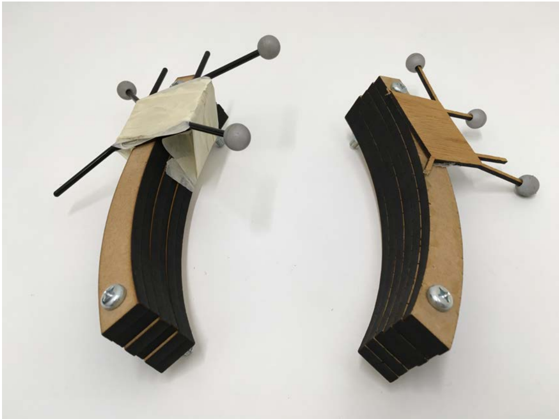
Figure 4.1: Free body joystick style steering wheel handles
